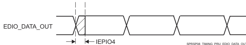
图 6-106. PRU_ICSSG PRU IEP Digital IOs Timing
