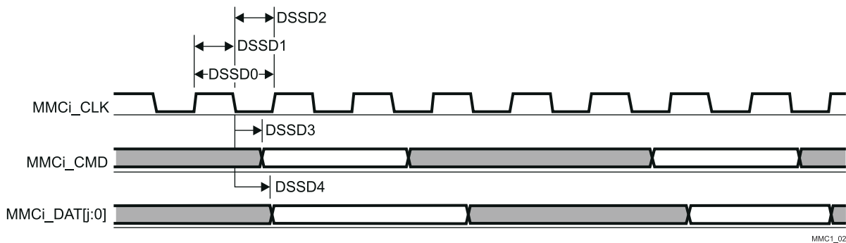
図 6-73. eMMC/SD/SDIO in - Default Speed - Transmitter Mode
