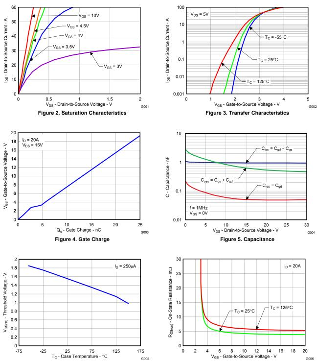
Figure 7. On-State Resistance vs. Gate-to-Source Voltage
