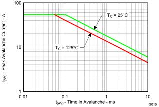
Figure 11. Single Pulse Unclamped Inductive Switching
