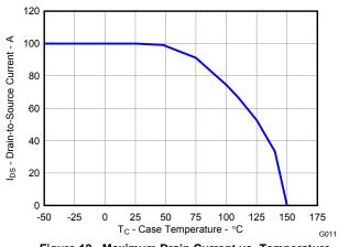
Figure 12. Maximum Drain Current vs. Temperature
