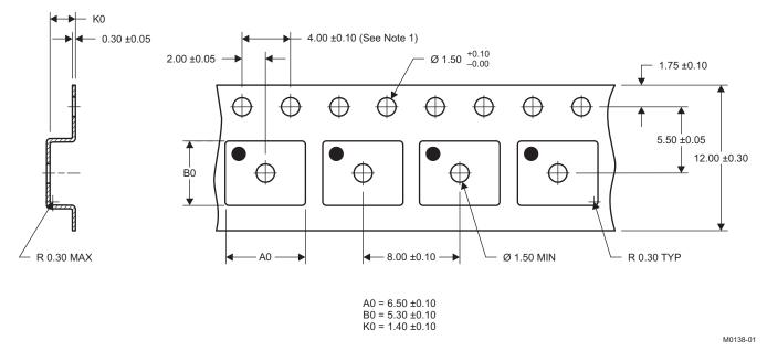
NOTES: 1. 10-sprocket hole-pitch cumulative tolerance ±0.2
