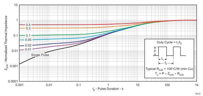
Figure 1. Transient Thermal Impedance
