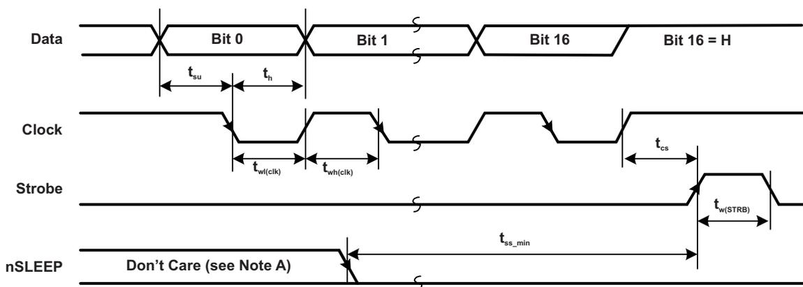
A. For initial setup, nSleep state can be "Don't care" before the t<sub>ss\_min</sub> timing prior to the strobe.
