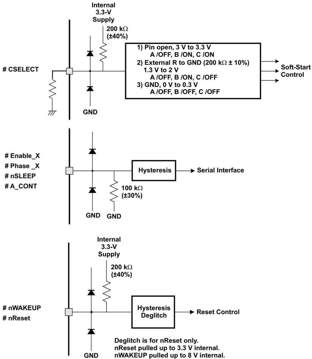
Figure 1. Input Pin Configuration
