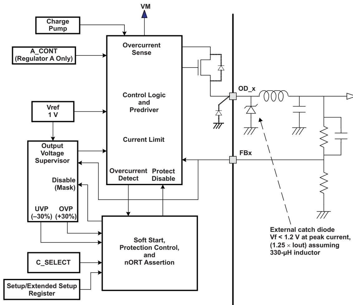
Figure 7. DC-DC Converter
