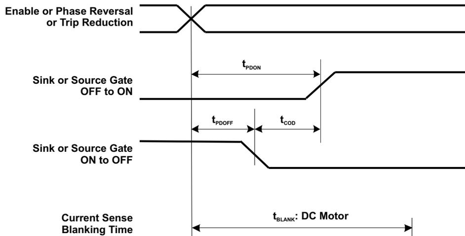
**Figure 6. Crossover and Blanking Timing for H-Bridge**
