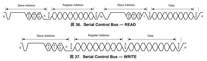
The I2C master located in the deserializer must support I2C clock stretching. For more information on I2C interface requirements and throughput considerations, refer to the *I2C Communication Over FPD-Link III with Bidirectional Control Channel* (SNLA131).
