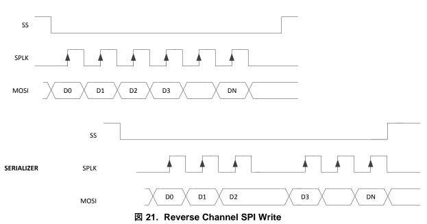
For reverse channel SPI reads, the SPI master must wait for a round-trip response before generating the sampling edge of the SPI clock. This is similar to operation in forward channel mode. Note that at most one data/clock sample is sent per back channel frame.
