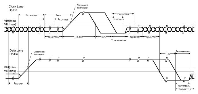
図 12. Switching the Clock Lane Between Clock Transmission and Low-Power Mode
