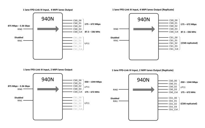
28. Data-Path Configurations with 1-Lane FPD-Link III Input
