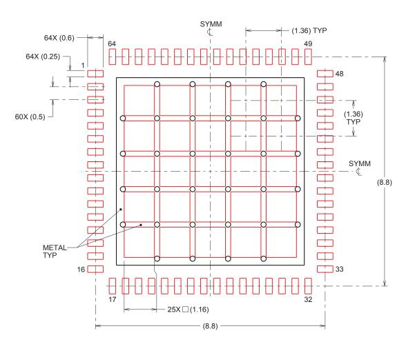
図 46. 64-Pin WQFN Stencil Example of Via and Opening Placement (Dimensions in mm)
