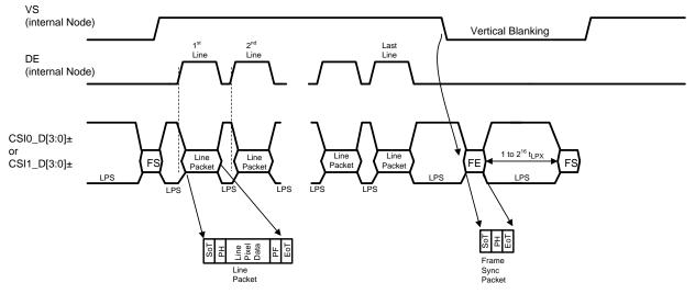
図 13. Long Line Packets and Short Frame Sync Packets
