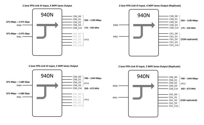
29. Data-Path Configurations with 2-Lane FPD-Link III Inputs
