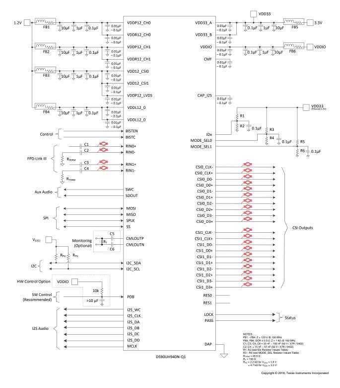
図 39. Typical Connection Diagram (Coax)
