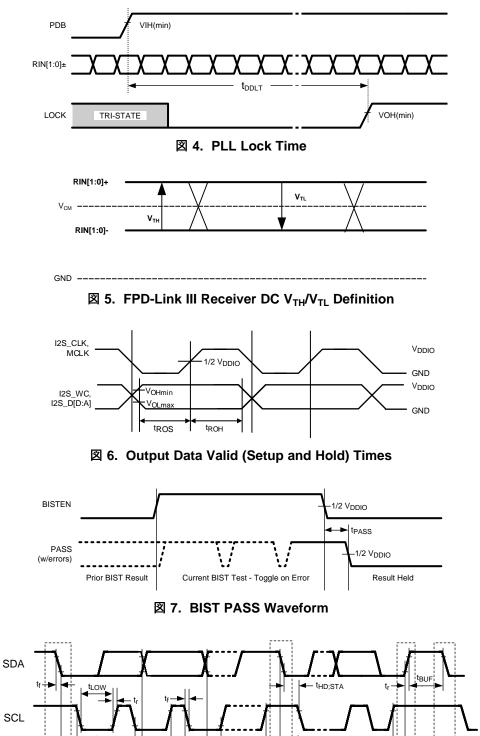
**8.** Serial Control Bus Timing Diagram
