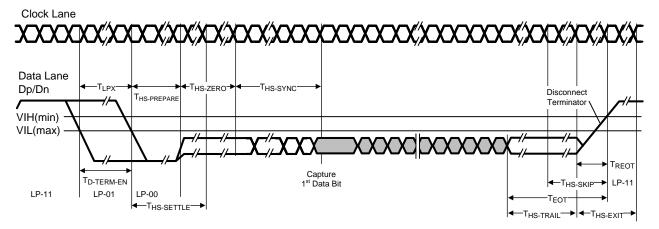
図 11. High-Speed Data Transmission Burst
