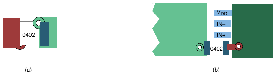
Figure 21. Typical Decoupling Capacitor Layouts
