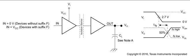
A.  $C_L = 15pF$  and includes instrumentation and fixture capacitance within  $\pm 20\%$ .
