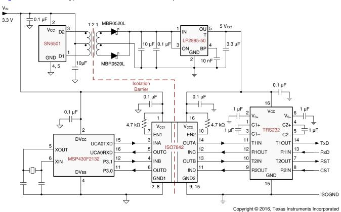
Figure 7-1. Isolated RS-232 Interface
