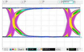
Figure 7-3. Eye Diagram at 100Mbps PRBS, 5V and 25°C
