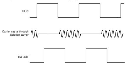
Figure 6-2. On-Off Keying (OOK) Based Modulation Scheme
