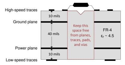
Figure 9-1. Layout Example Schematic
