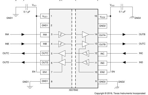
Figure 7-2. Typical ISO7842 Circuit Hook-Up
