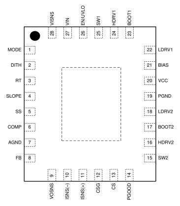
図 5-1. QFN-28 RHF Package Top View
