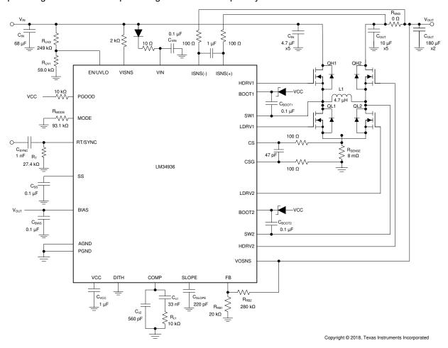
図 8-1. LM34936 Four-Switch Buck Boost Application Schematic
