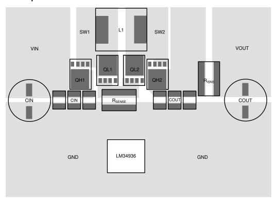
図 10-1. LM34936 Power Stage Layout
