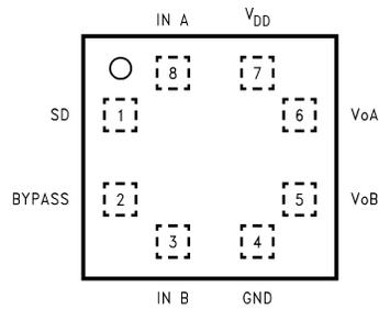
Figure 2. WQFN Package – Top View
