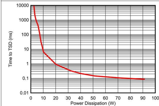
6-24. Time to Thermal Shut-Down During Inrush State
