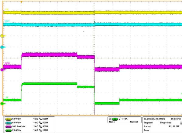
$V_{IN} = 12\text{ V}$ ,  $C_{OUT} = 22\ \mu\text{F}$ ,  $R_{IMON} = 1.15\ \text{k}\Omega$ ,  $I_{OUT}$  varied dynamically between 0 A and 3.5 A
