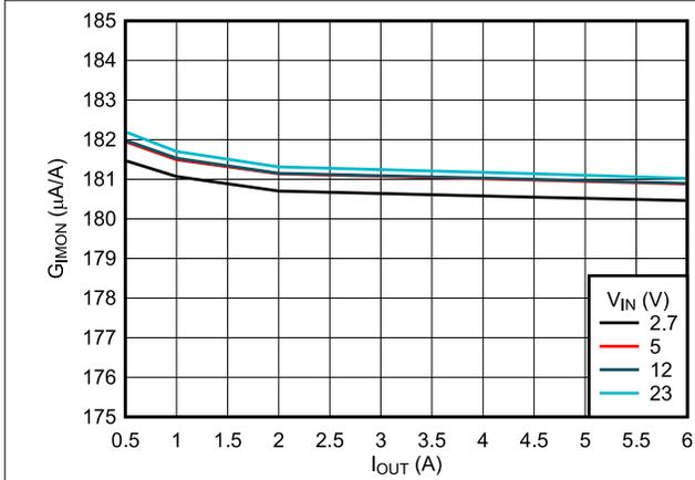
6-20. Analog Current Monitor Gain vs Load Current
