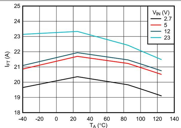
6-23. Steady State Fast-Trip Current Threshold vs Temperature
