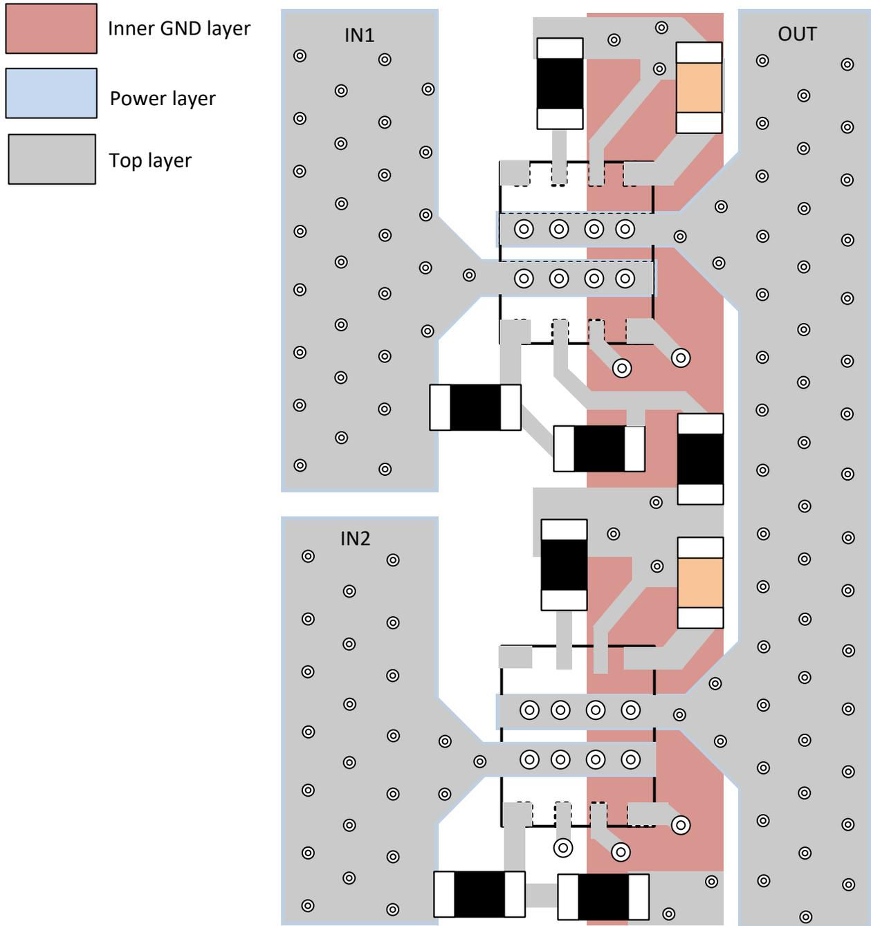
**10-2. Layout Example - 2 x LM73100 in ORing Configuration**
