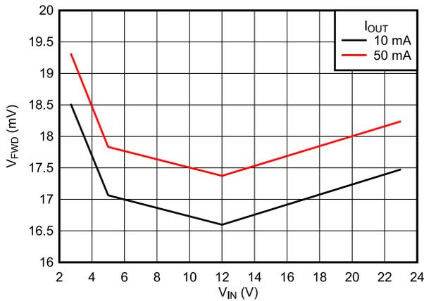
Figure 6-14. Forward Regulation Voltage vs Supply Voltage
