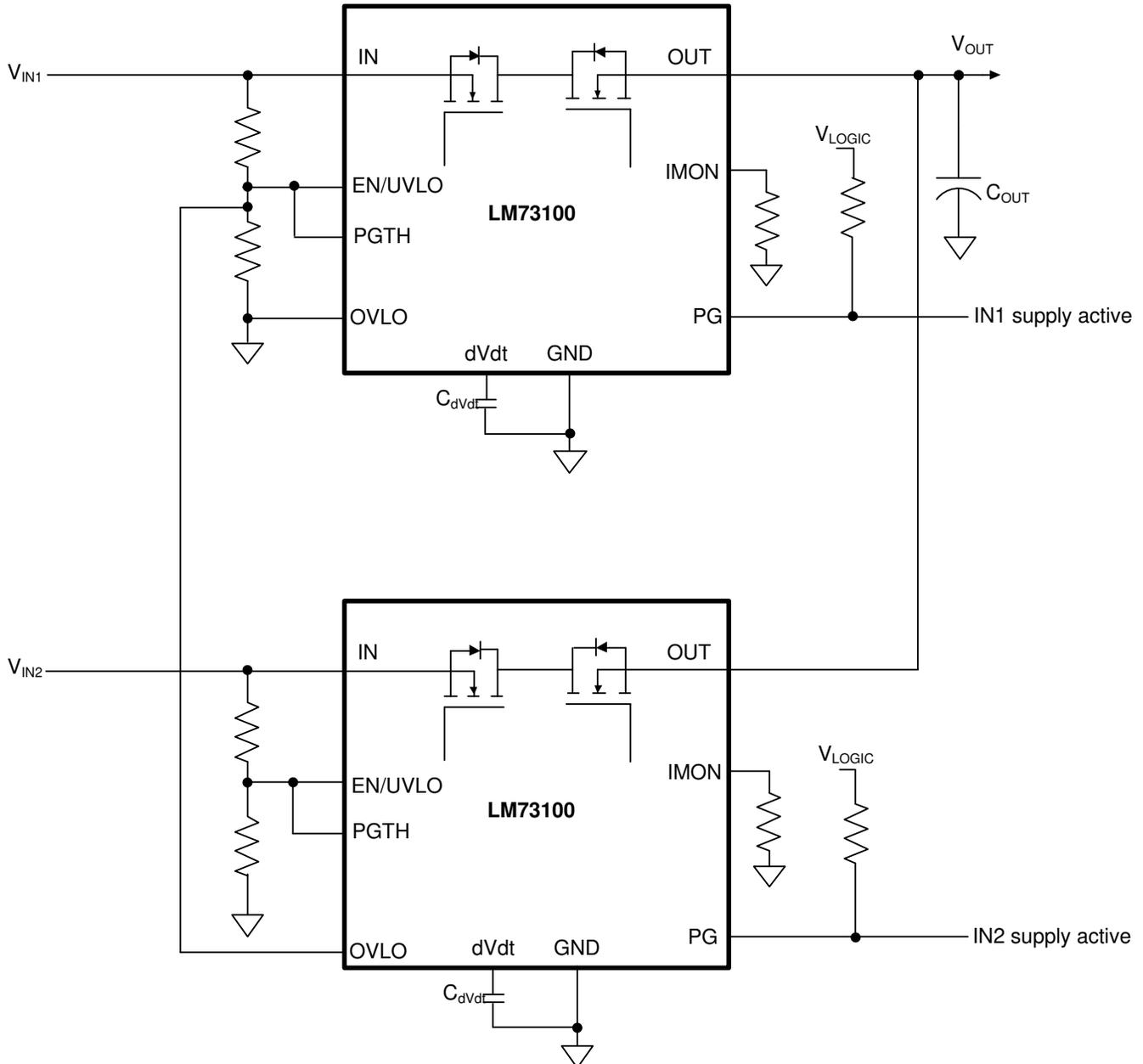
**图 8-10. Two Devices, Priority Power MUX Configuration**
