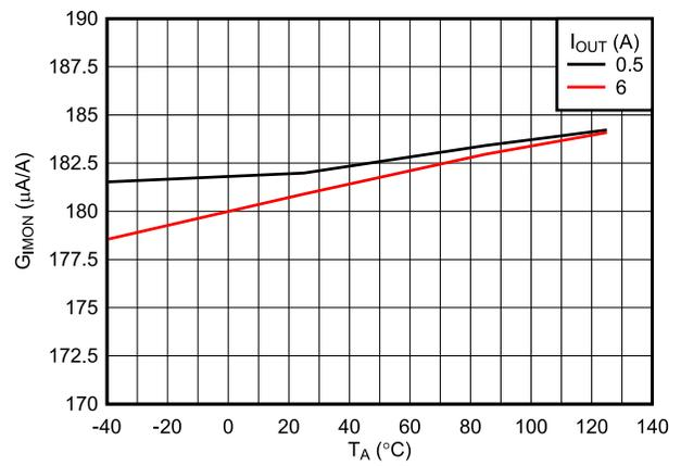
Figure 6-19. Analog Current Monitor gain vs Temperature
