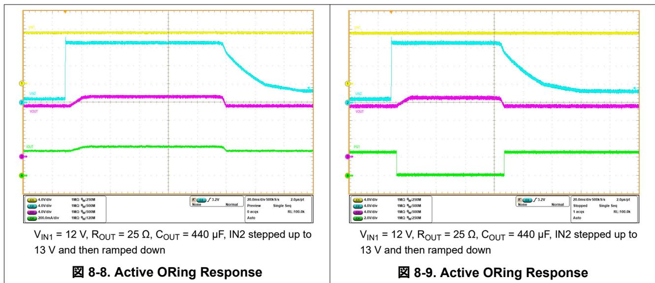
When bus voltages (IN1 and IN2) are matched, device in each rail sees a forward voltage drop and is ON delivering the load current. During this period, current is shared between the rails in the ratio of differential voltage drop across each device.
