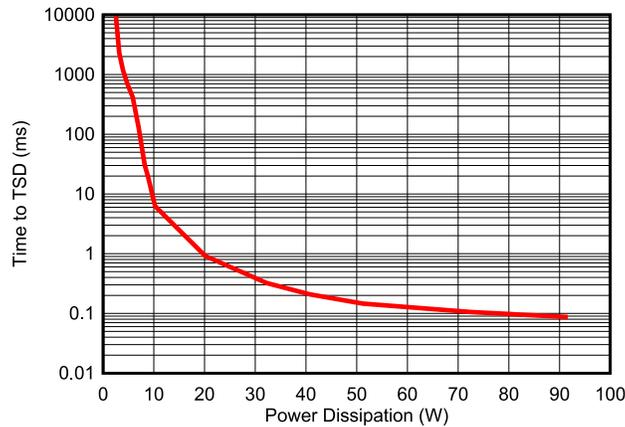
**8-3. Thermal shut-down plot during inrush**
