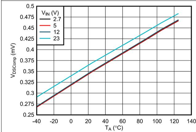
6-22. Steady State Fast-Trip Comparator Threshold vs Temperature
