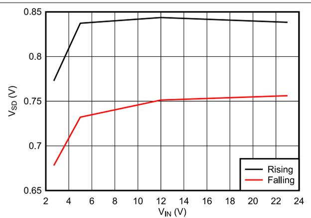
Figure 6-9. EN/UVLO Shutdown Threshold vs Supply Voltage
