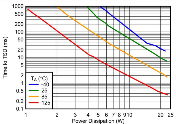
6-25. Time to thermal Shut-Down During Steady State
