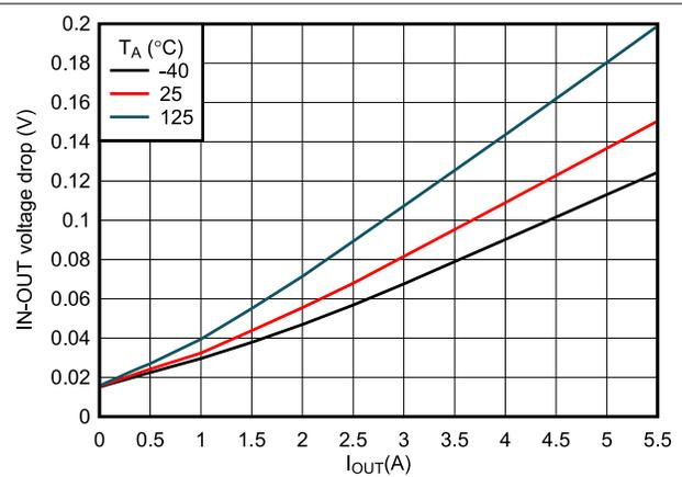
Figure 6-3. Forward Voltage Drop vs Load Current
