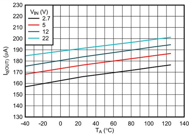
Figure 6-16. I<sub>OUT</sub> Leakage Current During ON-State Reverse Current Blocking
