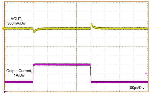
$V_{IN} = 12V$   $V_{OUT} = 3.3V$   $I_{OUT} = 1A$  to 3A
