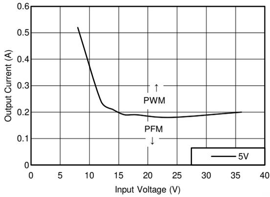
$V_{OUT} = 5\text{ V}$        $f_{SW} = 400\text{ kHz}$
