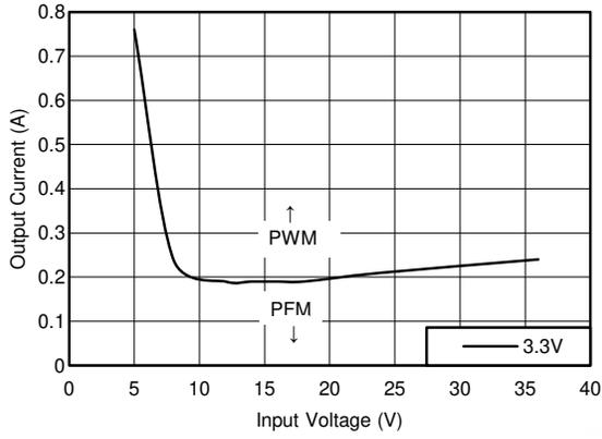
$V_{OUT} = 3.3V$   $f_{SW} = 400\text{ kHz}$
