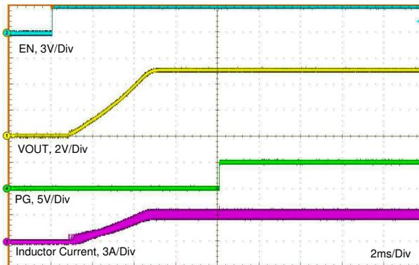
**8-4. Typical Start-Up Behavior  $V_{IN} = 12\text{ V}$ ,  $V_{OUT} = 5\text{ V}$ ,  $I_{OUT} = 3\text{ A}$**
