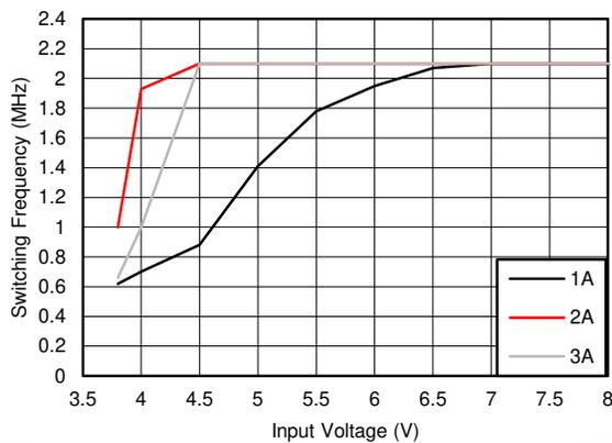
8-11. Typical Switching Frequency in Dropout
