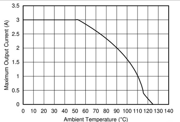
**Figure 9-4. Maximum Output Current vs Ambient Temperature**
