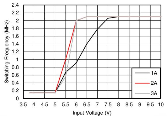
8-12. Typical Switching Frequency in Dropout
