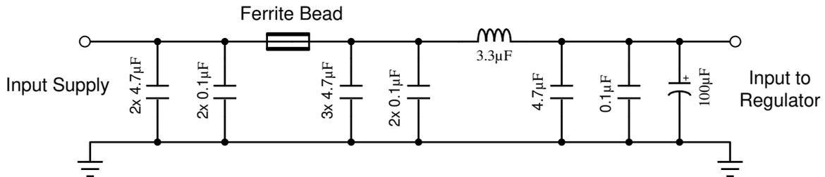
图 9-28. Typical Input EMI Filter
