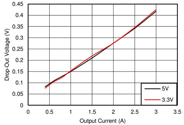
8-10. Typical Dropout Voltage vs Output Current
