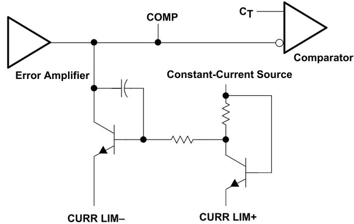
图 9-2. Current-Limit Schematic
