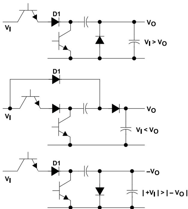
Figure 10-1. Capacitor-Diode-Coupled Voltage-Multiplier Output Stages
