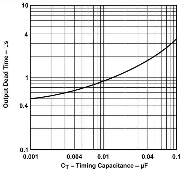
☒ 10-6. Output Dead Time vs Timing Capacitance
