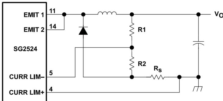
$$I_{O(\max)} = \frac{1}{R_s} \left( 200\text{ mV} + \frac{V_O R_2}{R_1 + R_2} \right)$$
