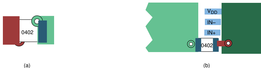
Figure 29. Typical Decoupling Capacitor Layouts
