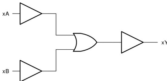
☒ 7-1. Logic Diagram, Each Gate (Positive Logic)
