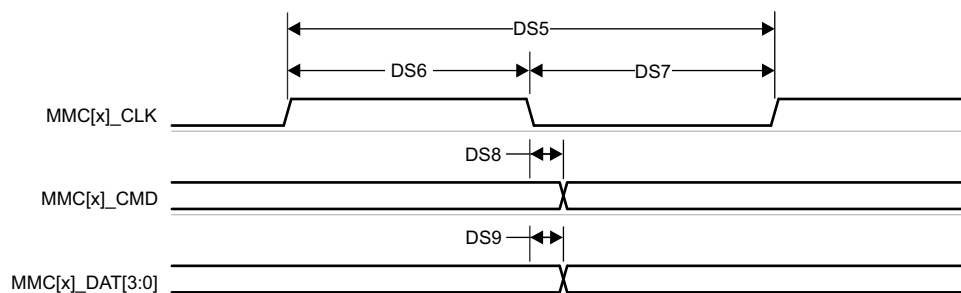
図 6-98. MMC1/2 – Default Speed – Transmit Mode
