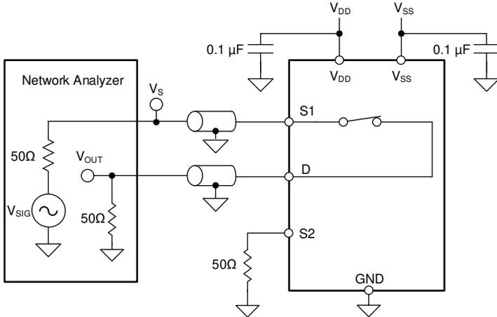
shows the setup used to measure bandwidth.
