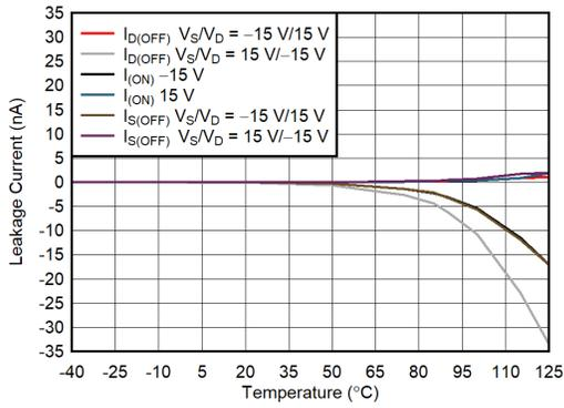
**6-9. Leakage Current vs Temperature**
