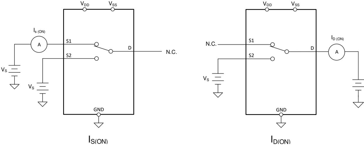
shows the circuit used for measuring the on-leakage current, denoted by  $I_{S(ON)}$  or  $I_{D(ON)}$ .
