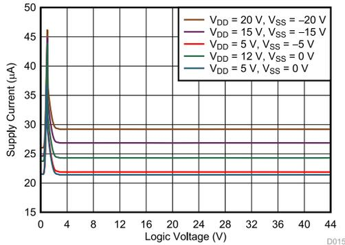
6-13. Supply Current vs Logic Voltage
