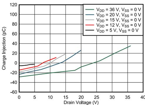
6-17. Charge Injection vs Drain Voltage – Single Supplies
