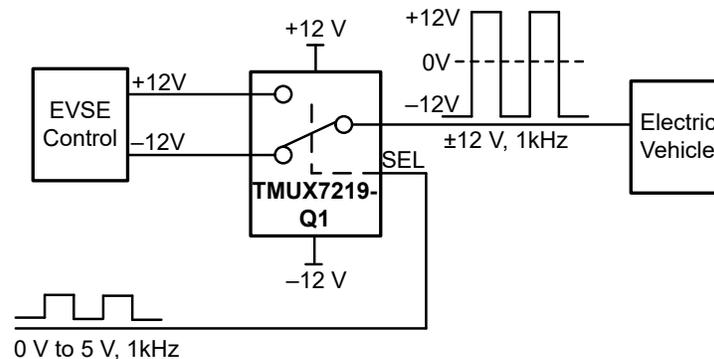
Figure 9-1. PWM Signal Generation (EV Charging Station)
