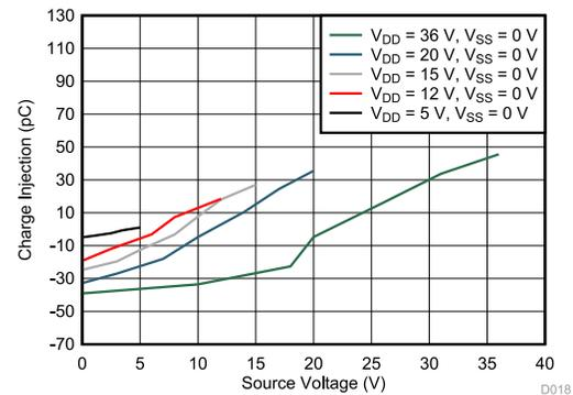
6-16. Charge Injection vs Source Voltage – Single Supplies
