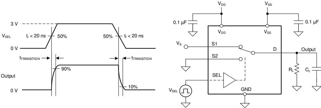
shows the setup used to measure transition time, denoted by the symbol  $t_{TRANSITION}$ .
