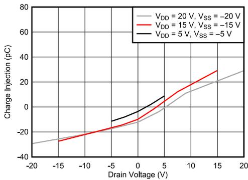
6-15. Charge Injection vs Drain Voltage – Dual Supplies
