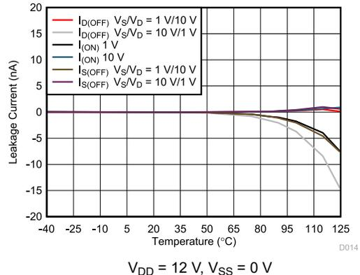
**6-12. Leakage Current vs Temperature**
