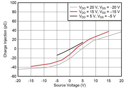
6-14. Charge Injection vs Source Voltage – Dual Supplies
