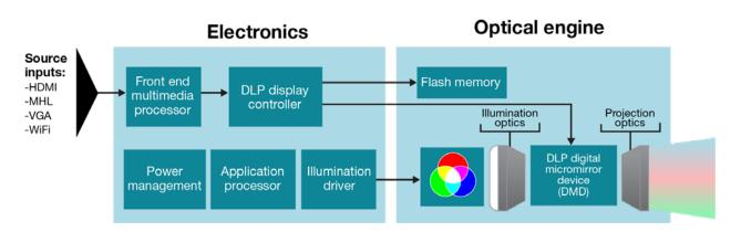
Figure 5. DLP Pico projection system block diagram.
