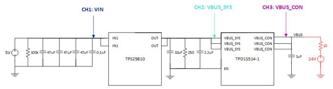
Figure 2. Test Configuration
