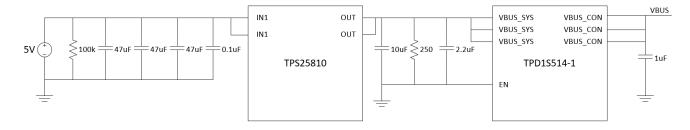
Figure 1. Overvoltage Protection Circuit
