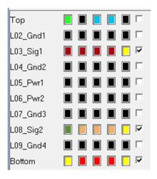
Board Stack-up Address/Command routed on layer 1, 2, 8 & 10
