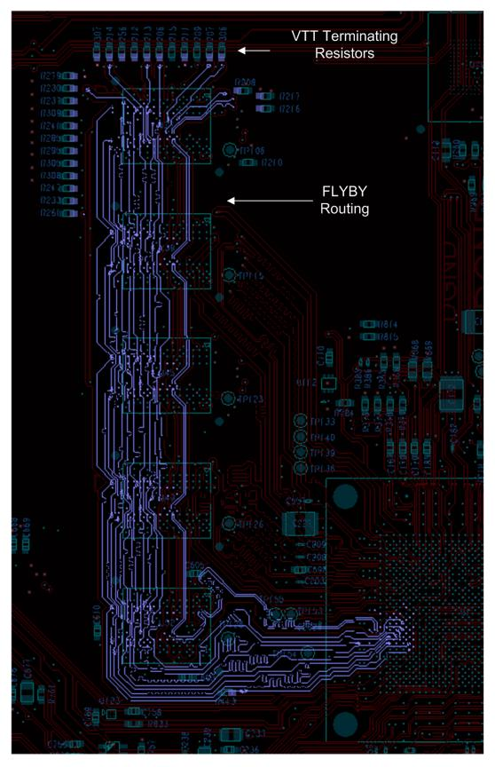
Figure 1-7. DDR3 Address/Command Group Flyby Routing
