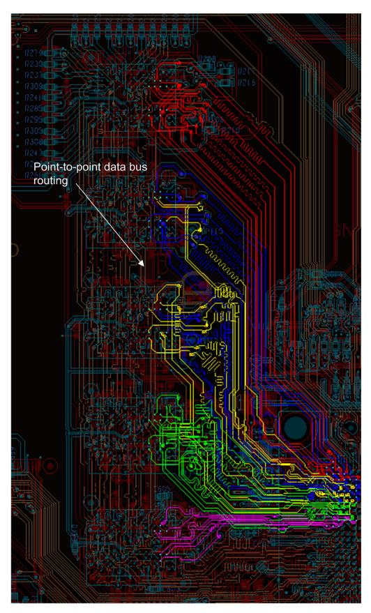
Figure 1-3. DDR3 Data Group Routing
