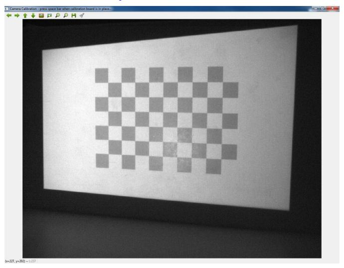
Figure 3-10. Camera Calibration Board Live View
