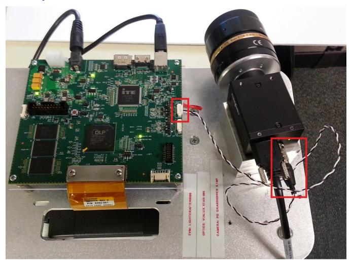
Figure 3-8. Connecting the Camera to the Host PC
