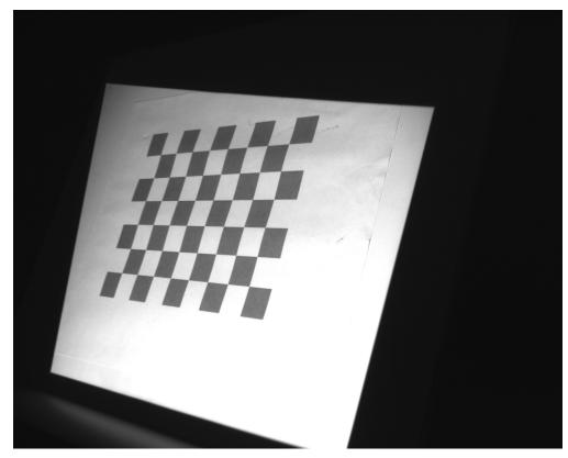
Figure 3-34. Projector Calibration Board Capture Position 9
