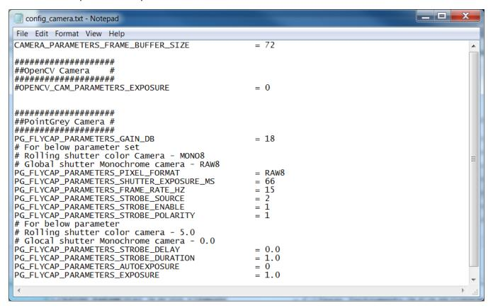
Figure 4-7. Camera Configuration File Settings for USB 2.0
