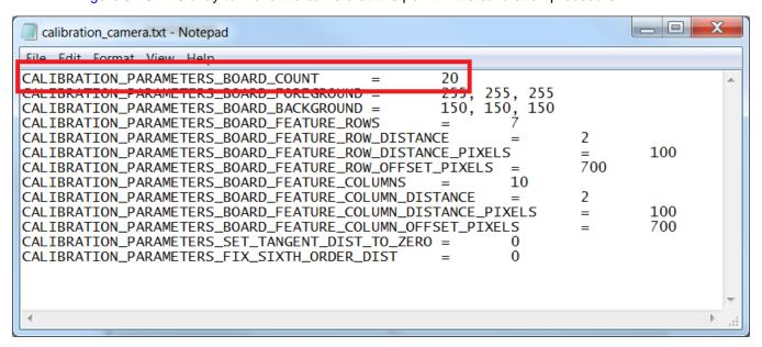
Figure 3-13. Camera Calibration Configuration File
