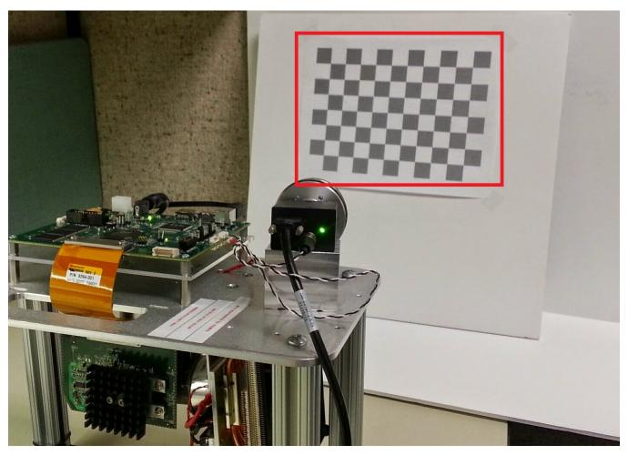
Figure 3-6. Calibration Board Attached to Flat Calibration Surface
