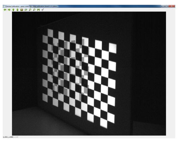
Figure 3-25. Projector Calibration Chessboard Capture
