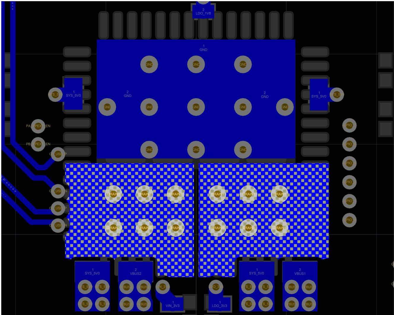
☒ 11-16. Figure 13. DRAIN1 and DRAIN2 Bottom Layer
