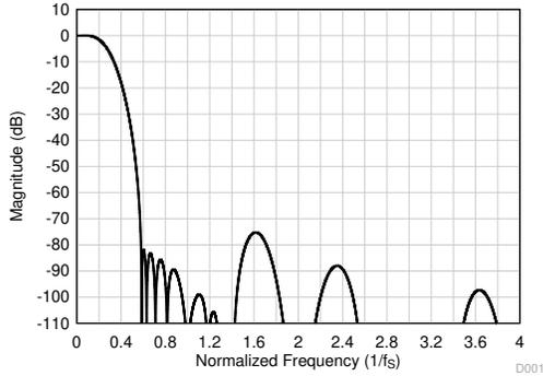
**图 8-35. Linear Phase Decimation Filter Magnitude Response**
