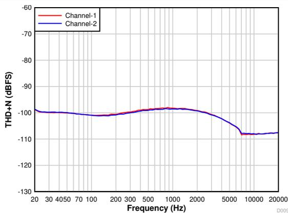
7-12. THD+N vs Input Frequency With a -1-dBr Input
