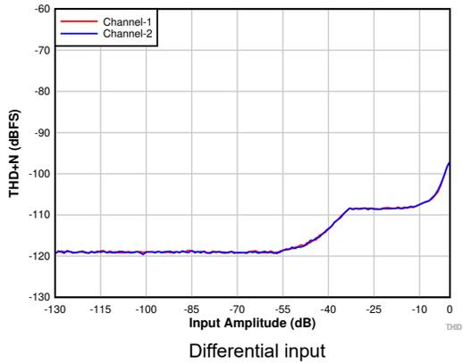
**7-4. THD+N vs Input Amplitude With DRE Enabled**
