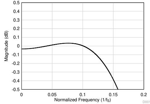
**图 8-36. Linear Phase Decimation Filter Pass-Band Ripple**
