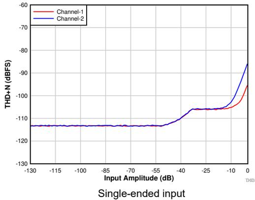
**7-6. THD+N vs Input Amplitude With DRE Enabled**
