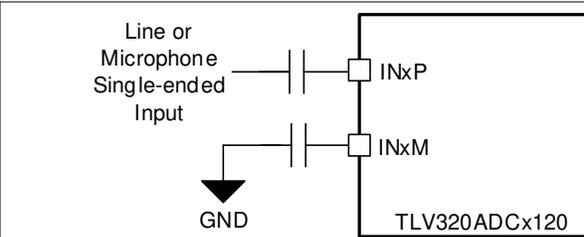
图 8-15. Single-Ended, AC-Coupled Input Connection
