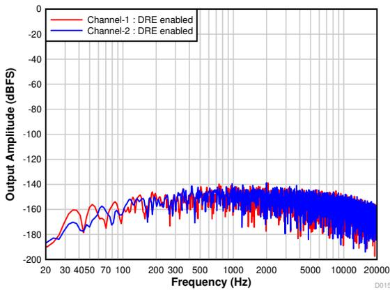
7-18. FFT With Idle Input With DRE Enabled
