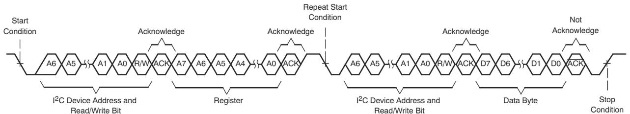
**Figure 8-69. I<sup>2</sup>C Single-Byte Read Transfer**
