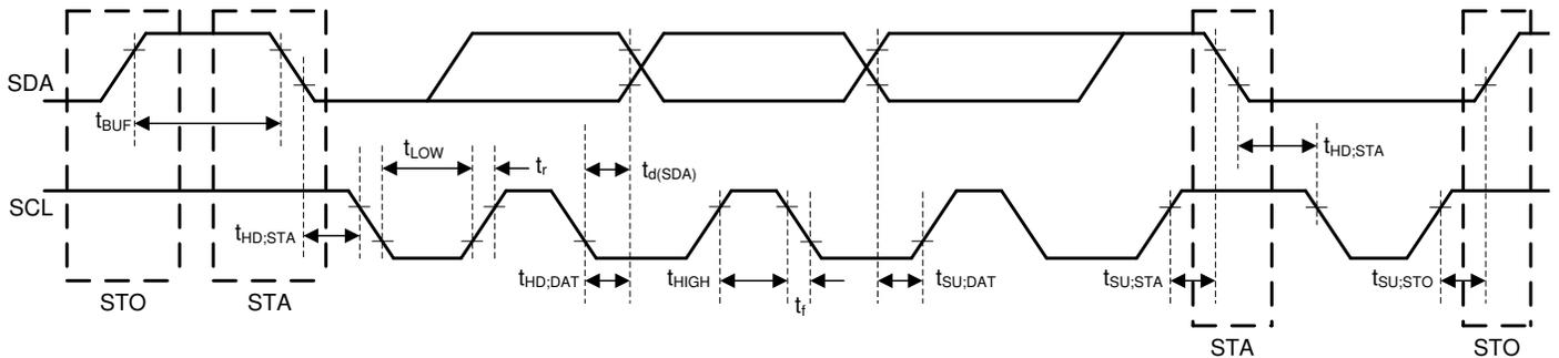
7-1. I<sup>2</sup>C Interface Timing Diagram
