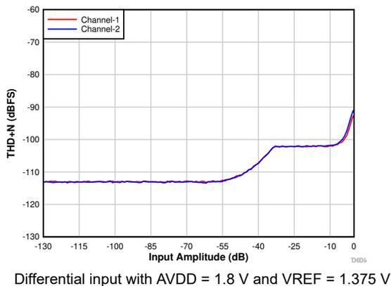
**7-8. THD+N vs Input Amplitude With DRE Enabled**
