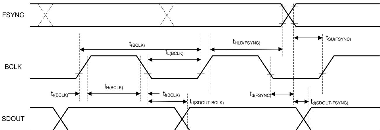
7-2. TDM (With BCLK\_POL = 1), I<sup>2</sup>S, and LJ Interface Timing Diagram
