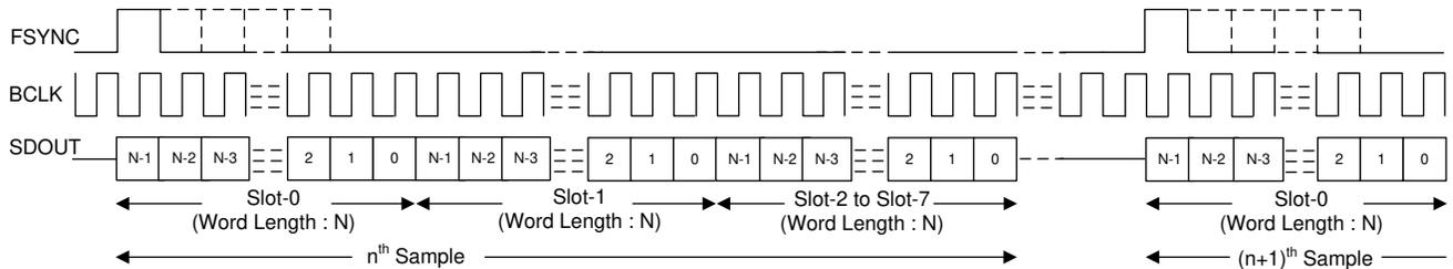
8-4. TDM Mode Protocol Timing (TX\_OFFSET = 0 and BCLK\_POL = 1)
