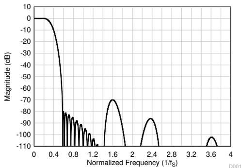
图 8-33. Linear Phase Decimation Filter Magnitude Response
