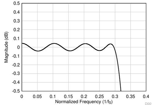
图 8-32. Linear Phase Decimation Filter Pass-Band Ripple
