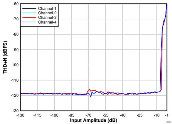
7-24. PDM Input THD+N vs Input Amplitude
