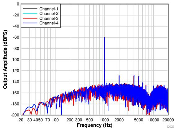
7-26. PDM Input FFT With a -60-dBr Input
