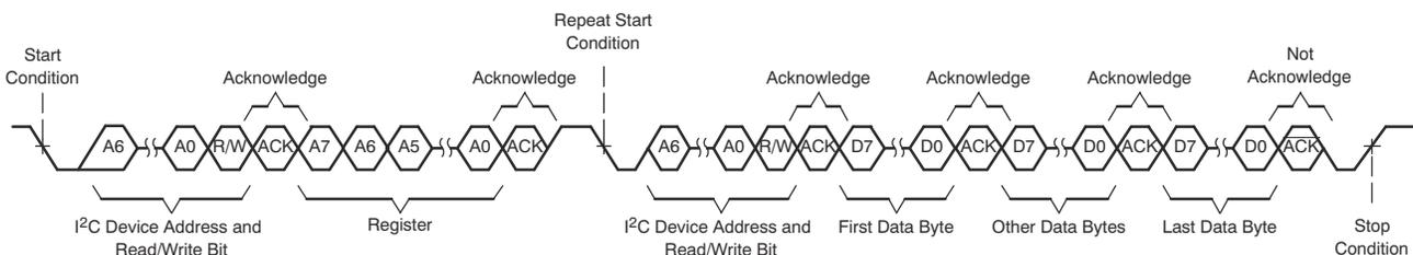
**Figure 8-70. I<sup>2</sup>C Multiple-Byte Read Transfer**
