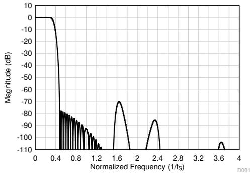
图 8-31. Linear Phase Decimation Filter Magnitude Response
