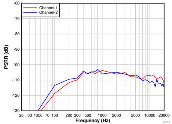
7-17. Power-Supply Rejection Ratio vs Ripple Frequency With 100-mV<sub>pp</sub> Amplitude
