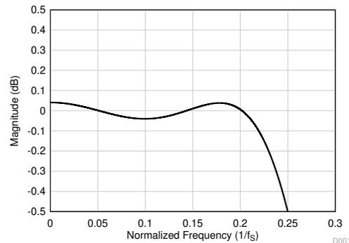
图 8-34. Linear Phase Decimation Filter Pass-Band Ripple
