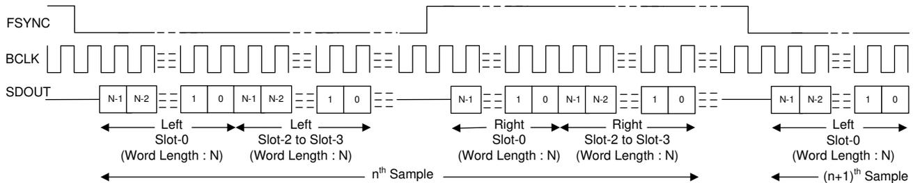
8-5. I<sup>2</sup>S Mode Standard Protocol Timing (TX\_OFFSET = 0)
