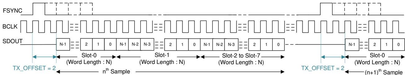
**图 8-2. TDM Mode Protocol Timing (TX\_OFFSET = 2)**
