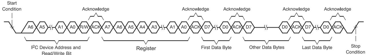
**Figure 8-68. I<sup>2</sup>C Multiple-Byte Write Transfer**
