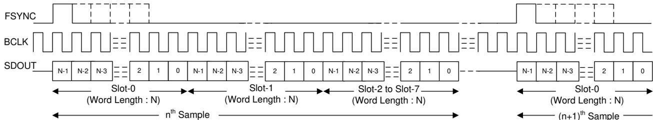
**图 8-1. TDM Mode Standard Protocol Timing (TX\_OFFSET = 0)**
