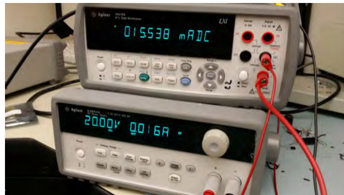
Figure 22. Power Supply and Multimeter Connected in Series
