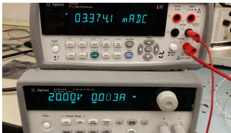
Figure 23. Default Current Drawn by the System When the Firmware is Not Programmed
