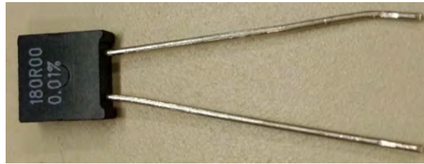
Figure 39. Precision Resistors 0.01% Tolerance Used for ADC Characterization
