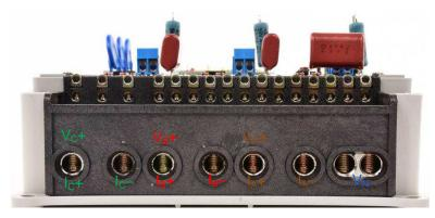
図 23. Front View of EVM With Test Setup Connections With Current and Voltage Connected
