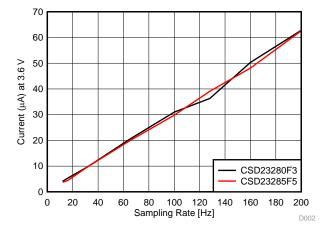
**図 10.** Power Consumption Comparison for Two FemtoFET Devices
