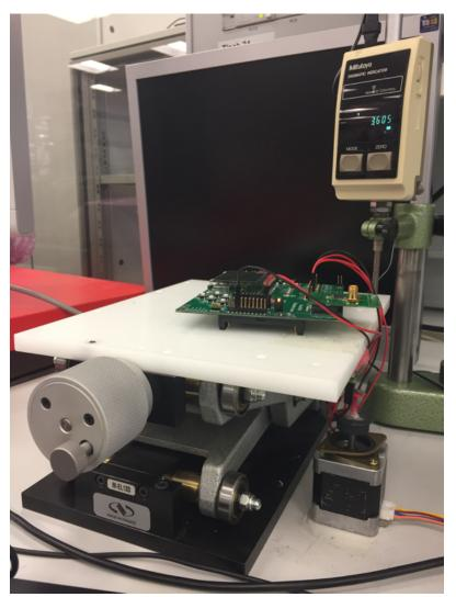
図 8. Stepper Motor With Disc at 3.6-mm Distance From TIDA-01228 (Face Down)
