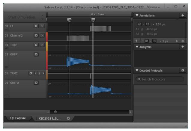
図 7. Undampened LCsensor1 and LCsensor2 Oscillation With Approximately 500 kHz Each
