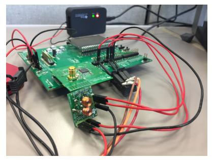
☑ 9. SRF06EB Wiring for EnergyTrace Measurements With FET430 Pro
