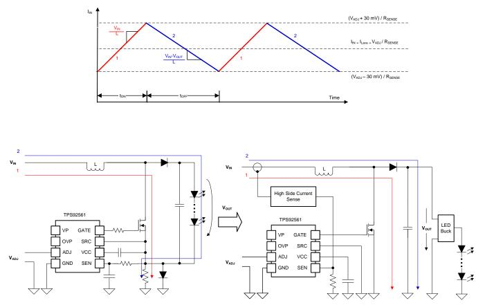
図 33. Pre-Boost Operation—Standard vs Modified Implementation and Input Current Waveform
