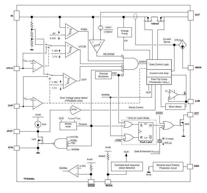
図 4. Functional Block Diagram of TPS2660x
