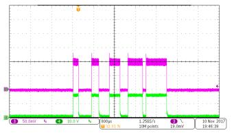
$\boxtimes$  49. Time Bracketing: On Time = 400  $\mu s,$  Frame Rate = 1428 Hz, N = 5,  $I_{\text{LED}}$  = 1000 mA, Time Brk = 0.5
