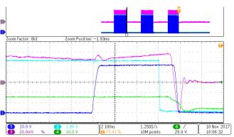
$\boxtimes$  61. LED Buck Normal Operation Control Through BUCK\_ON Signal, LED ON/OFF—Transition During  $t_{\text{on}}$
