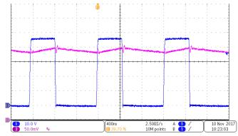
37. Buck Switch Node at 2400 mA of LED Current
