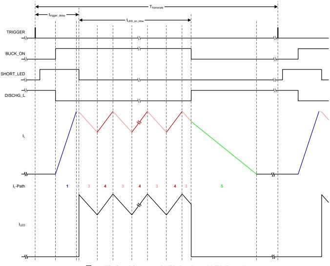
図 27. Timing Diagram of LED Buck and LED Board
