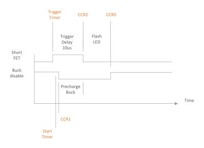
図 35. Timing of Buck Regulator and Short FET
