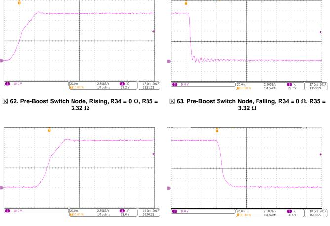
$\boxtimes$  64. Pre-Boost Switch Node, Rising, R34 = 15 Ω, R35 =  $\boxtimes$  65. Pre-Boost Switch Node, Falling, R34 = 15 Ω, R35 = 15 Ω
