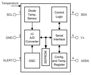
図 17. Functional Block Diagram of TMP116
