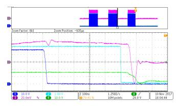
☑ 60. LED Buck Normal Operation Control Through BUCK\_ON Signal, LED ON/OFF—Transition During t<sub>orr</sub>
