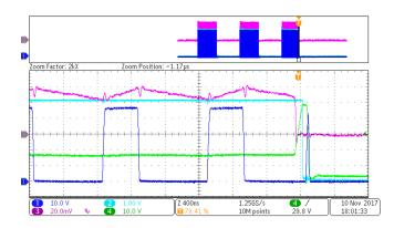
☑ 58. LED Buck OVP—Third LED Pulse Stopped After Overvoltage Caused by Removing SH-J5
