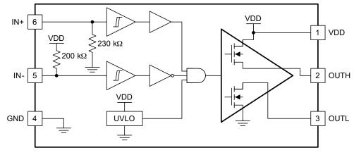
図 15. Functional Block Diagram of UCC27511
