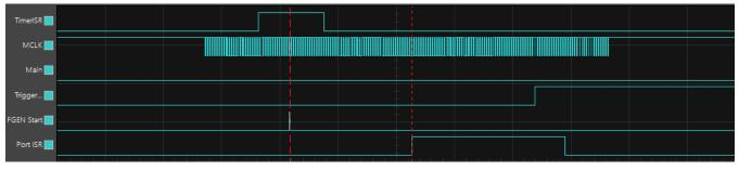
図 42. Jitter on External IRQ Caused by Timer (1 µs/div)
