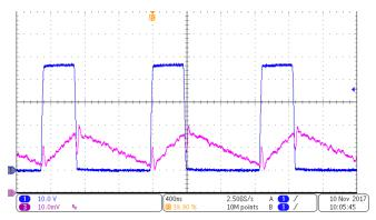
356. Buck Switch Node at 200 mA of LED Current
