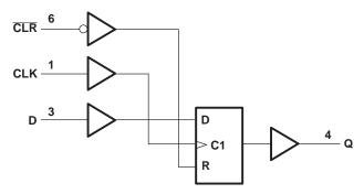
図 18. Functional Block Diagram of SN74LVC1G175
