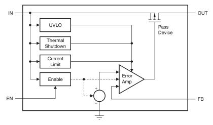
図 14. Functional Block Diagram of TPS7A4101
