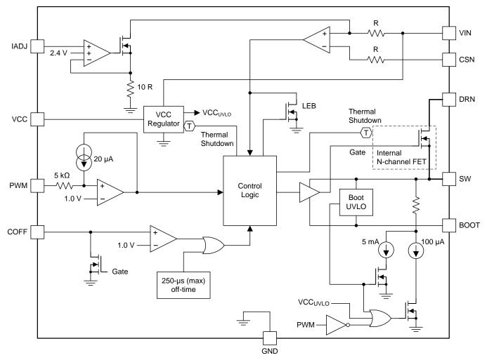
図 2. Functional Block Diagram of TPS92515HV
