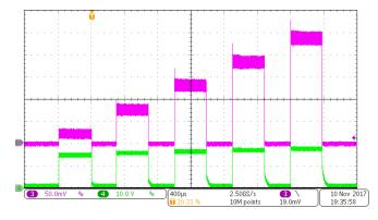
$\boxtimes$  48. Current Bracketing: On Time = 400 µs, Frame Rate = 1428 Hz, N = 5, I LED = 200 mA, Current Brk = 550 mA, 5 Steps From 200 mA to 2.4 A in 4 Increments of 550 mA
