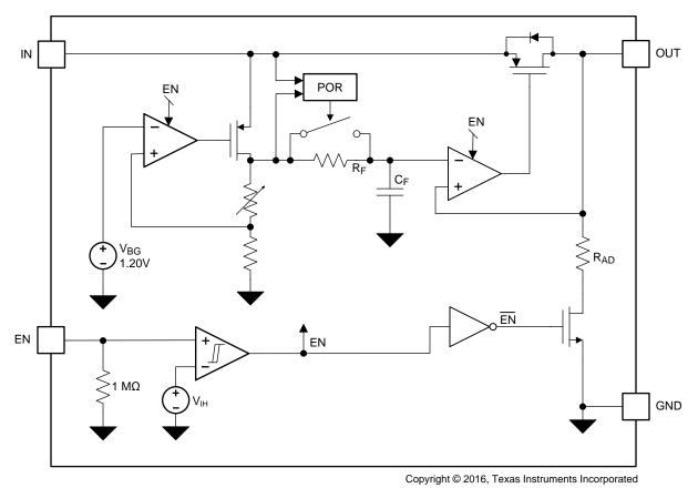
図 12. Functional Block Diagram of LP5907
