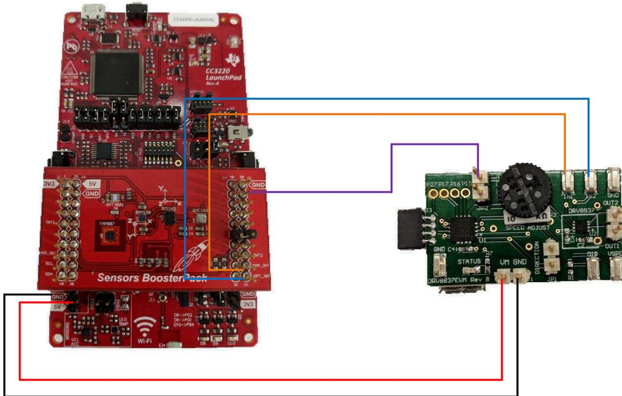
図 16. Jumper Wire Placement to Connect DRV8837EVM to System
