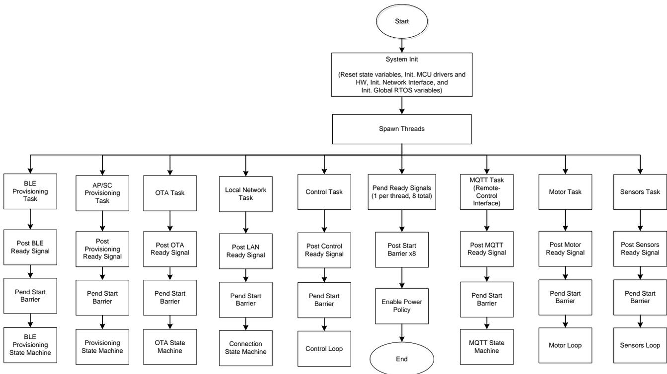
図 4. Overall Software Flow Diagram
