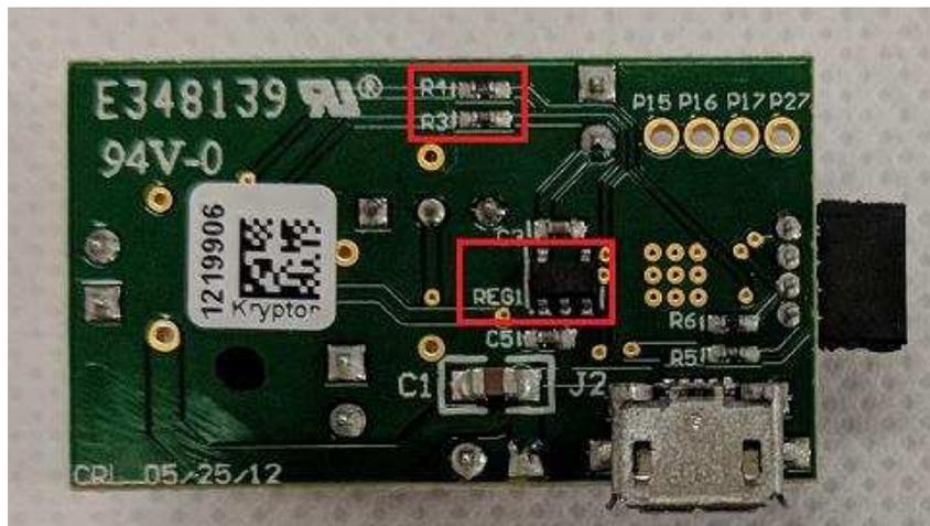
23. Back of DRV8837EVM With Components To Remove Highlighted
