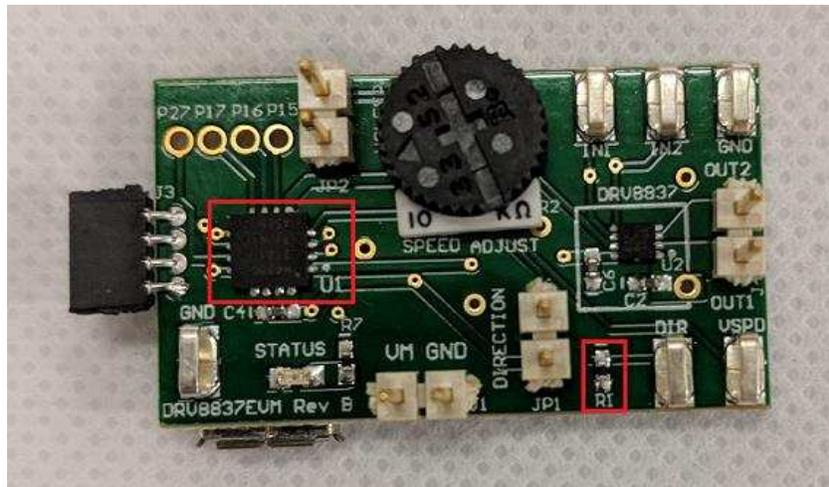
図 24. Front of DRV8837EVM With Highlighted Components To Remove
