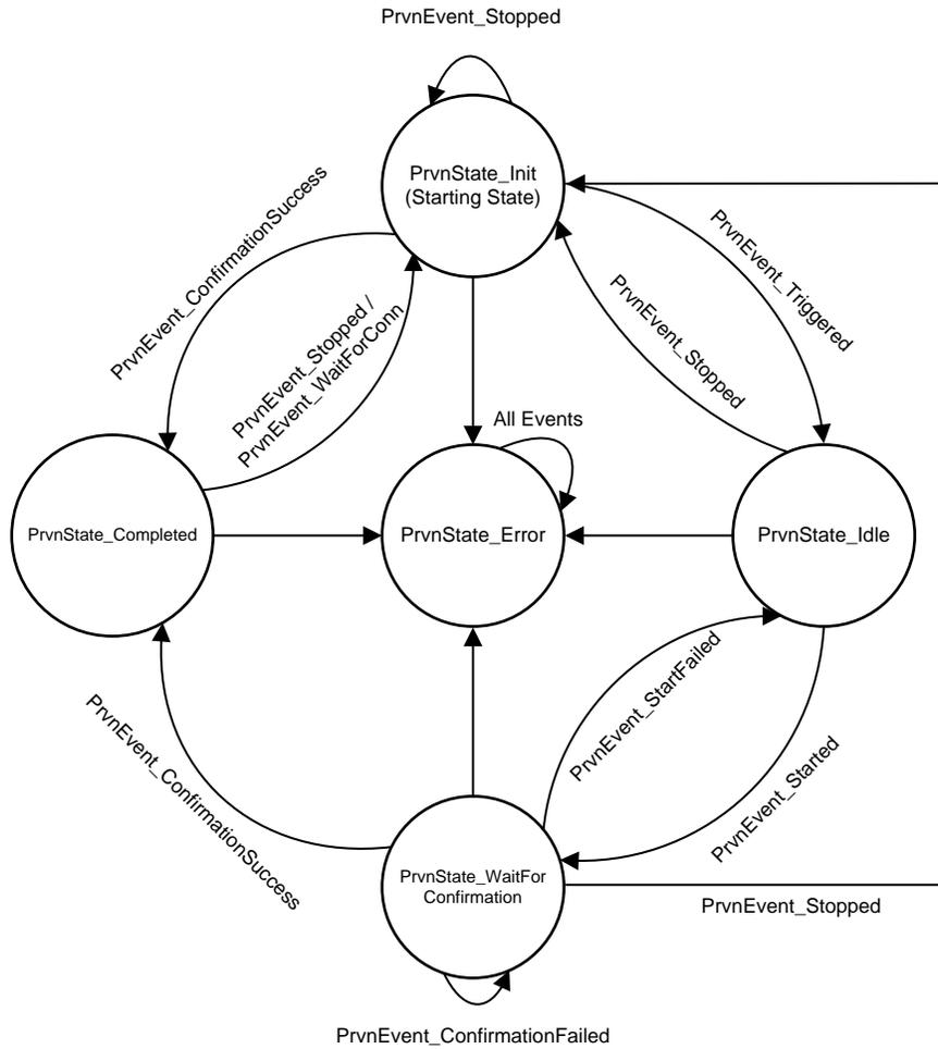
Figure 6. Provisioning Task State Machine
