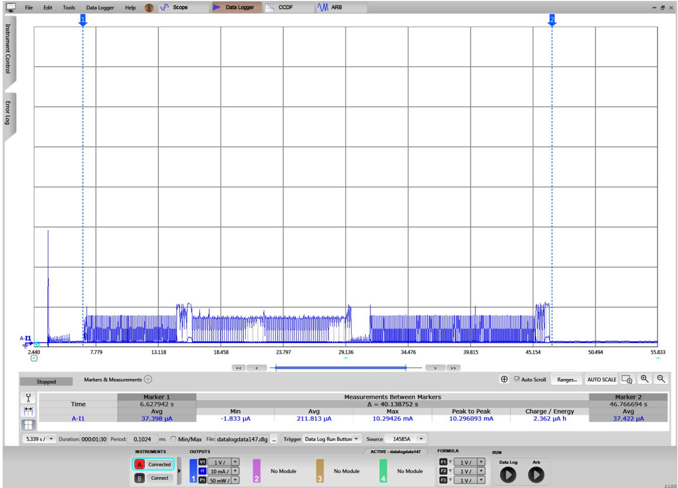
Figure 28. CC2640R2F Current Consumption During Provisioning
