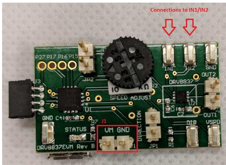
Figure 14. J1 and IN1/IN2 Highlighted on Front of DRV8837EVM
