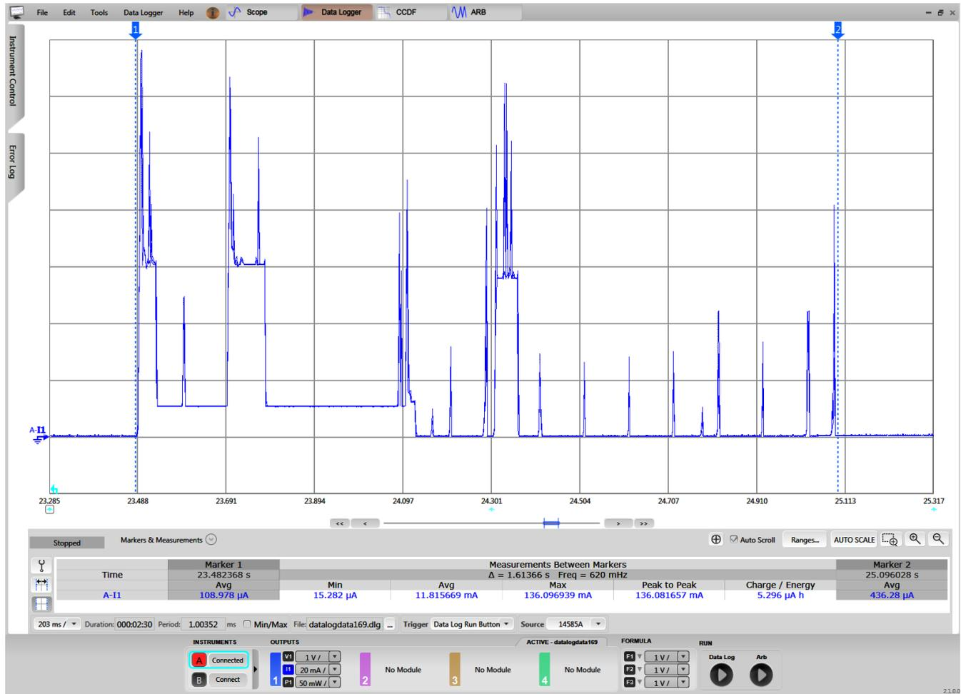
**Figure 27. CC3220 Current Consumption During Lock Status Request**
