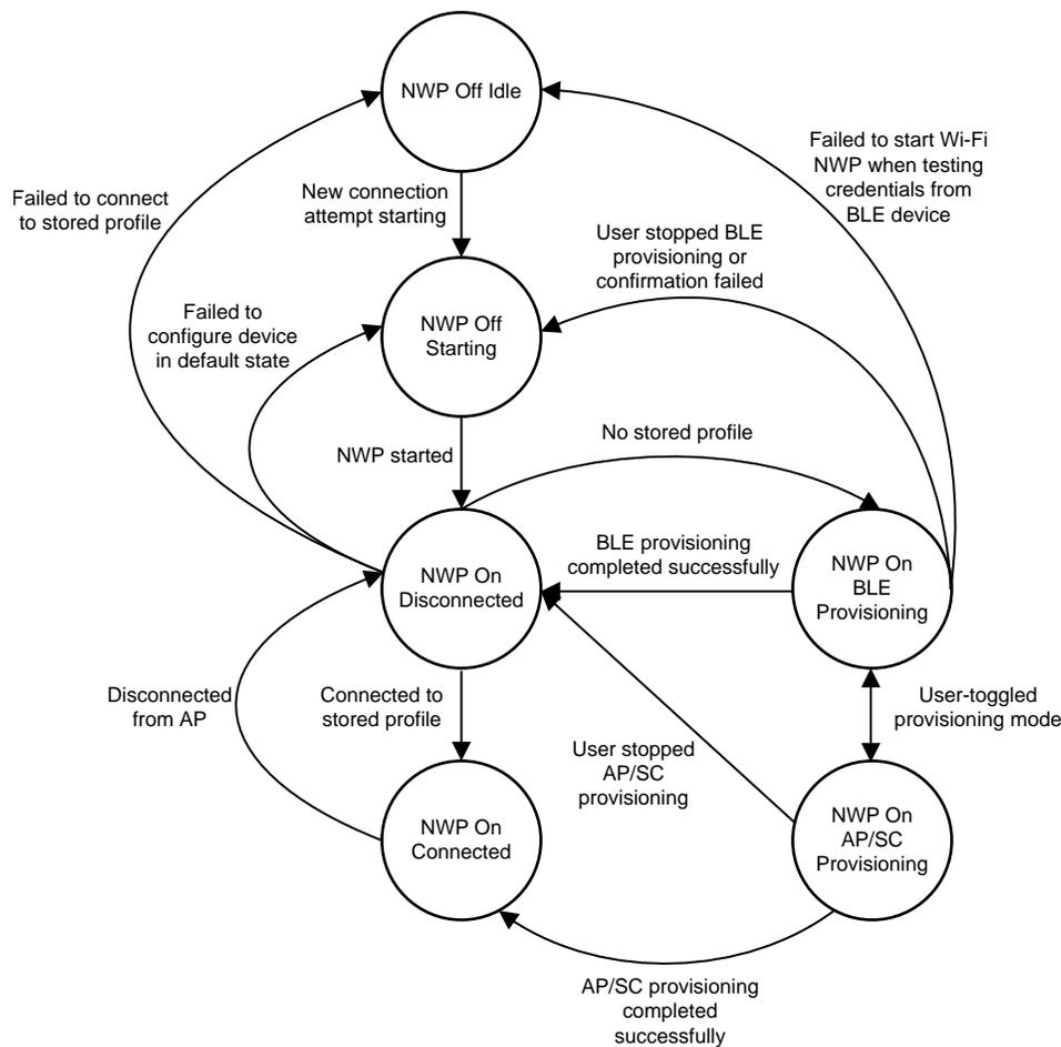
図 5. Network-Connection Management-Thread Flow Diagram
