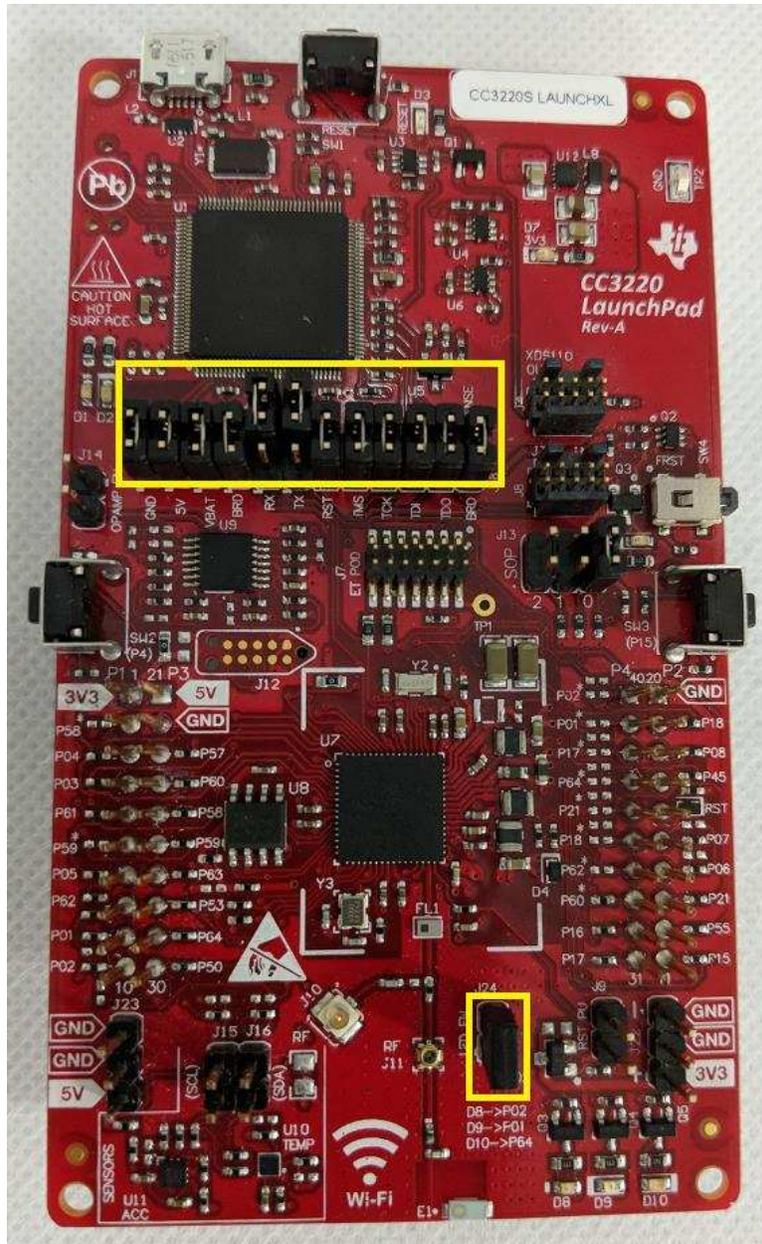
**Figure 11. CC3220S-LAUNCHXL Jumper Configuration**
