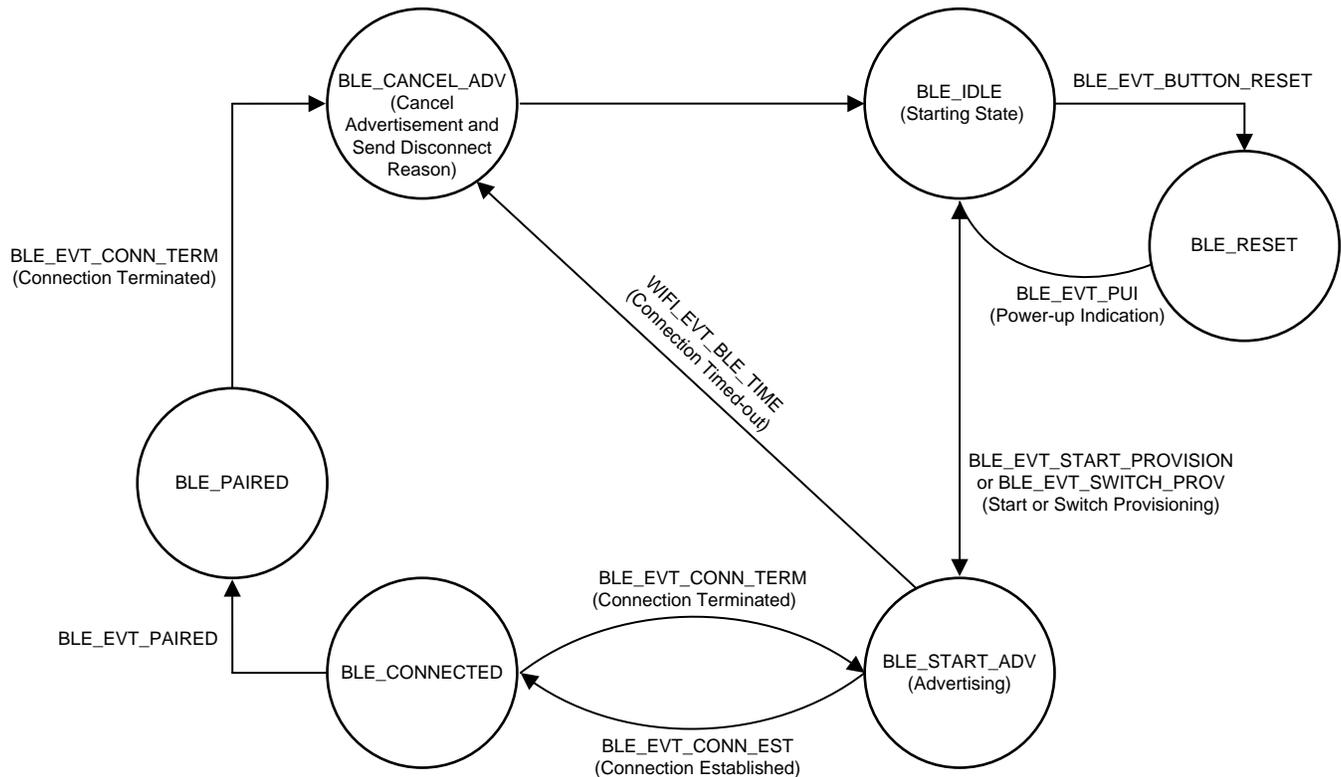
Figure 7. BLE Provisioning State Machine
