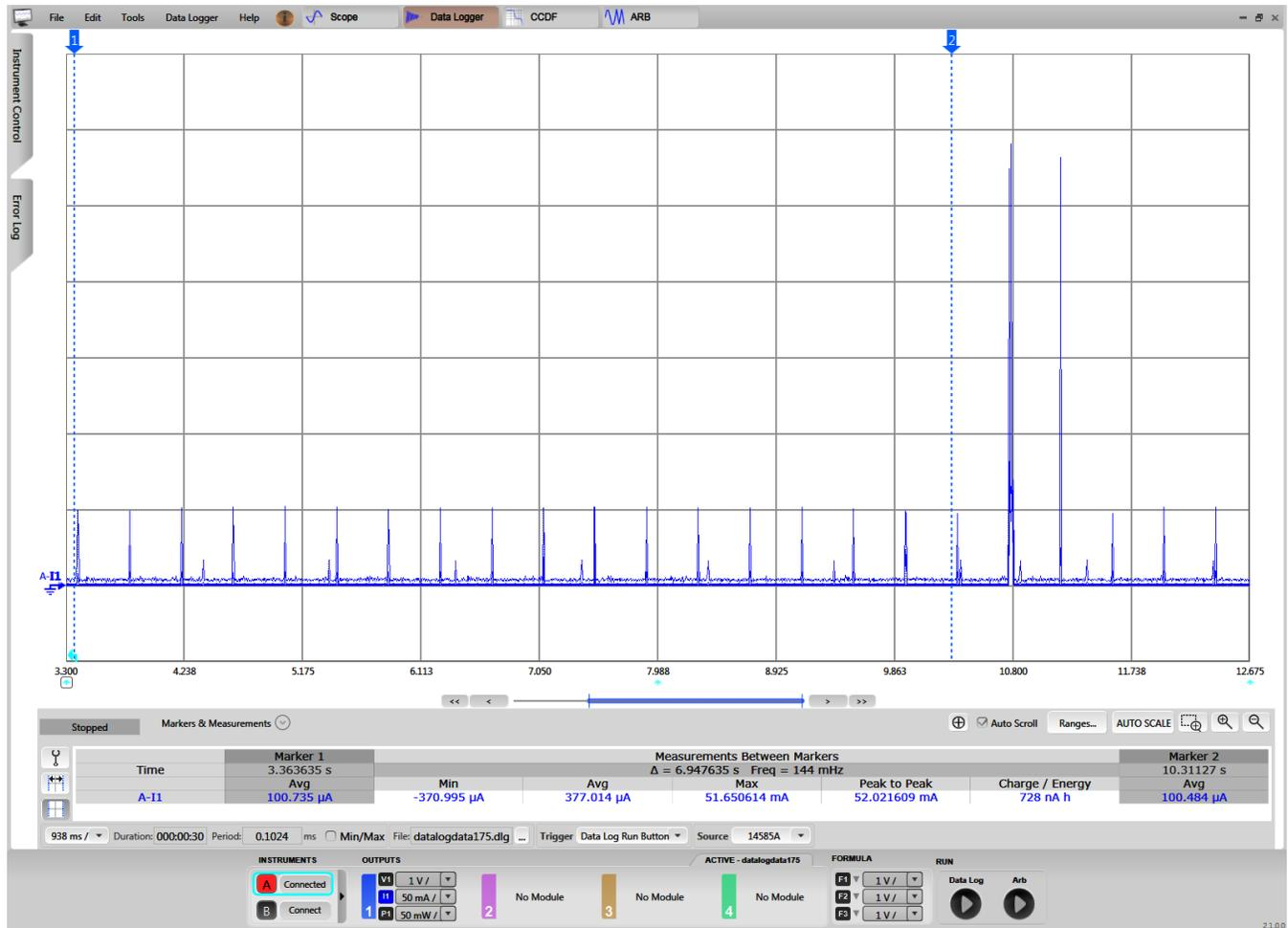
**Figure 25. CC3220S Current Consumption Versus Time While in Idle Connected Mode With 400-ms LSI**
