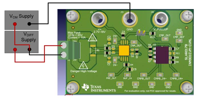
Figure 3. Supply Setup for Common and Differential Voltage
