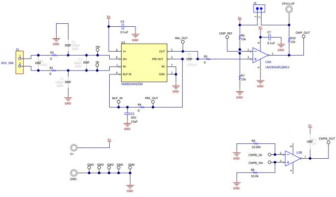
Figure 4. INA901EVM-CVAL Schematic
