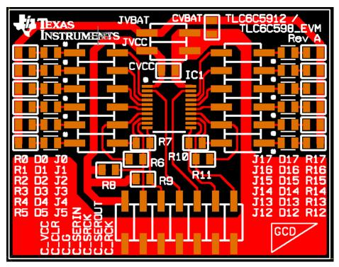
Figure 3. Top Assembly Layer
