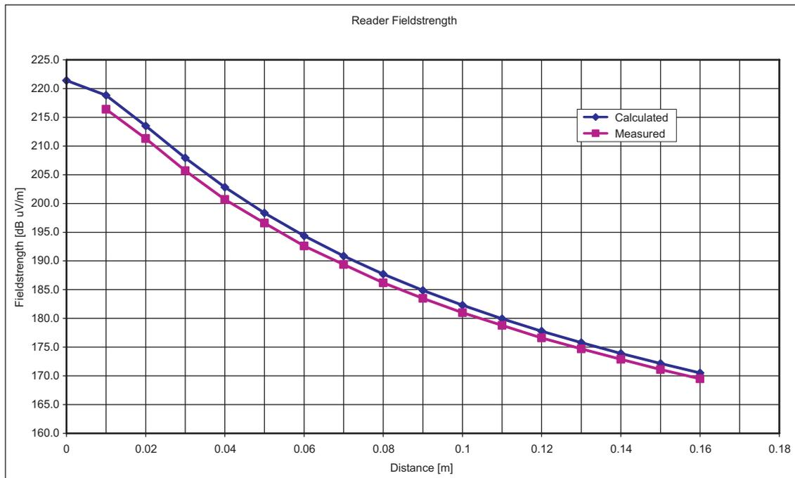
Figure 5. Calculated Reader Field Strength Over Distance
