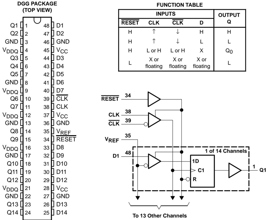
**Figure 3. Function Table, Pinout, and Logic Diagram of the SSTV16857**
