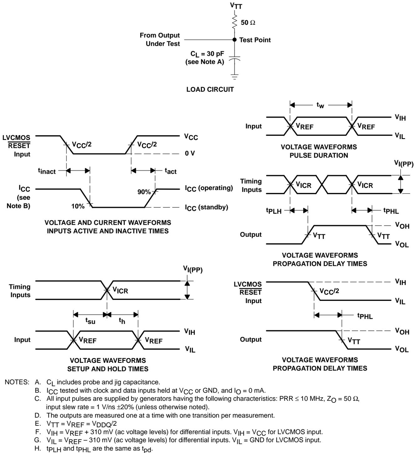
Figure 9. SSTV16857 Load Circuit and Voltage Waveforms
