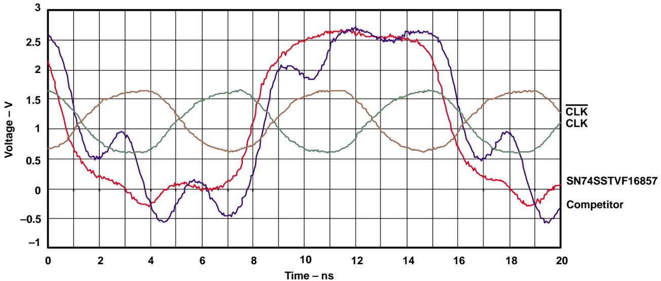
**Figure 6. Single-Bit (Q2 Output) Switching Results on Raw Card Version B RDIMM**
