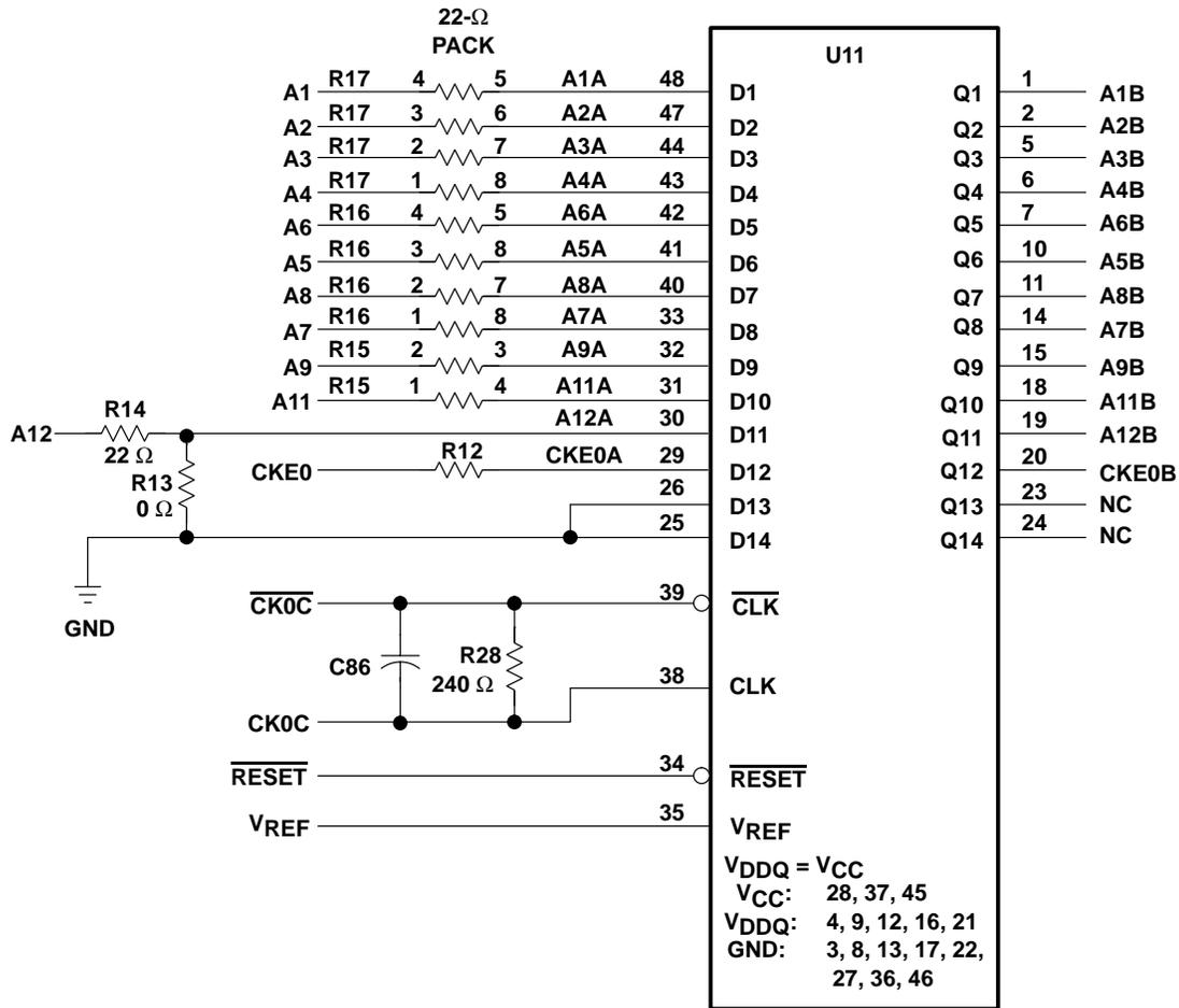
Figure 5. SSTV16857 (U11) as Connected on the Raw Card Version B DDR RDIMM
