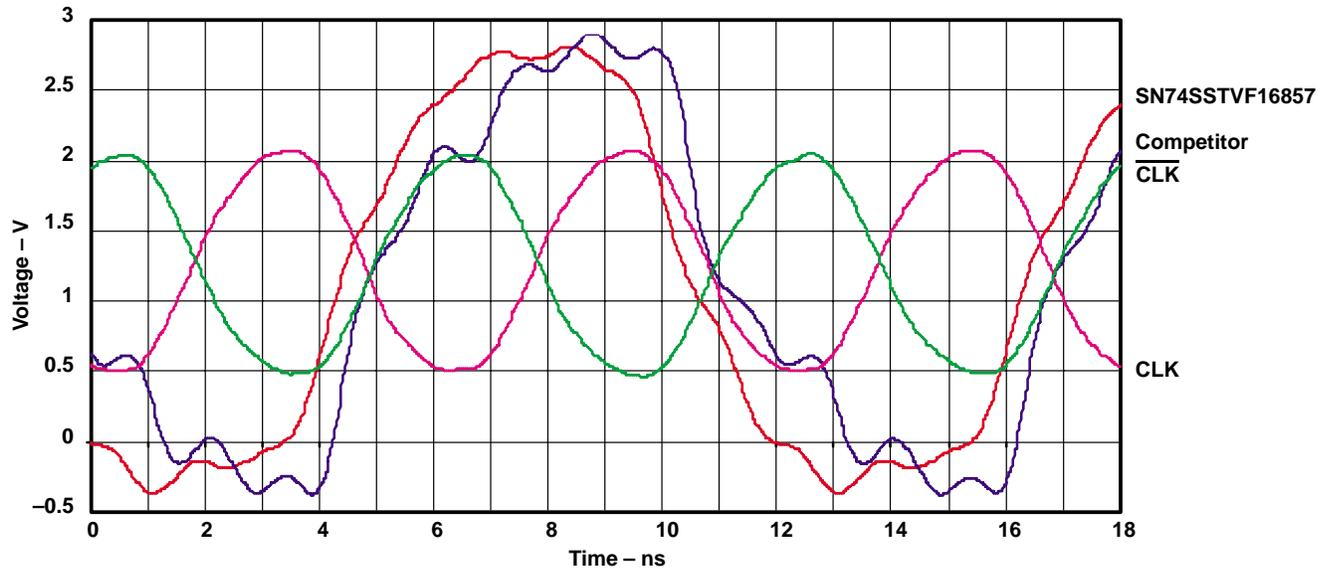
**Figure 7. Q2 Output Switching In-Phase (Synchronously) With Ten Other Outputs**
