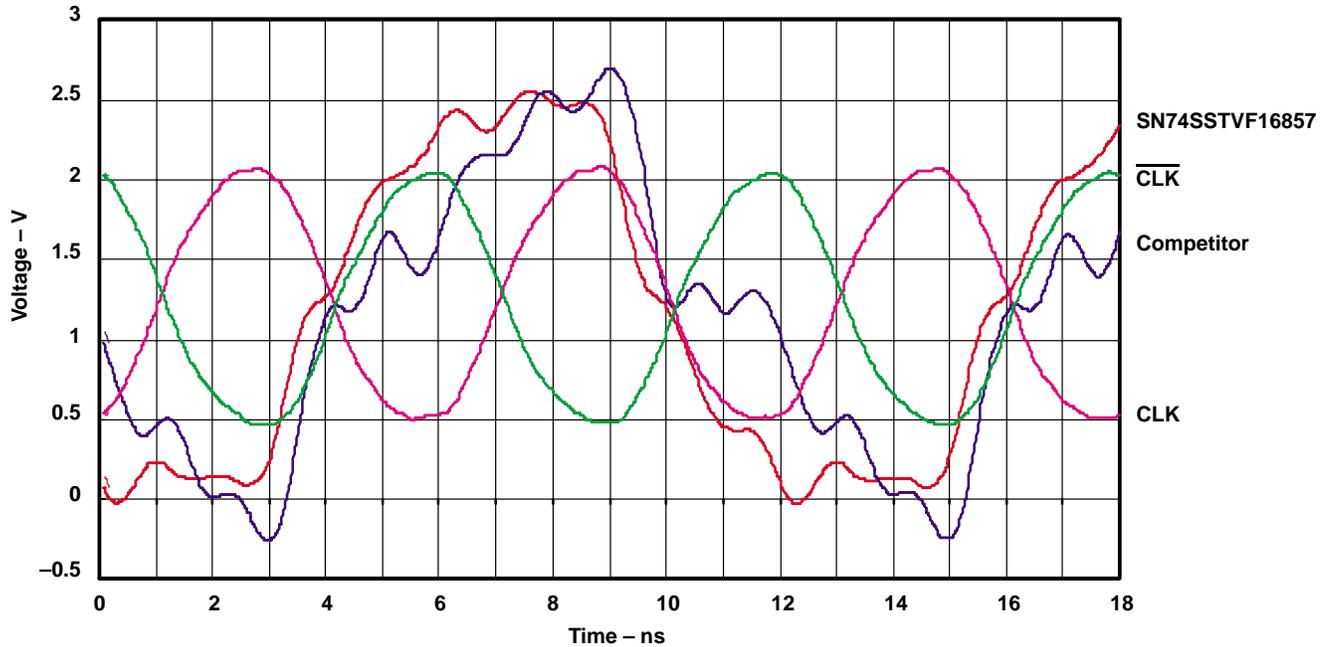
**Figure 8. Q2 Output Switching Out-of-Phase (Complementarily) with Ten Other Outputs**
