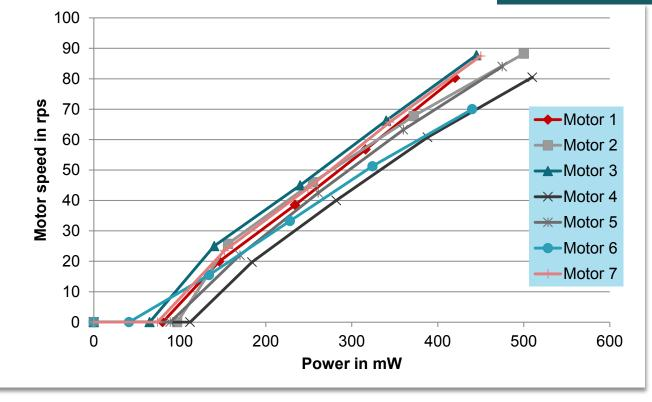
Power = Voltage\*Current\*DutyCycle
