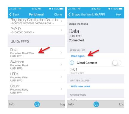
You can write the characteristic by clicking "Write new value". Writing a new value will open a dialog window, into which you type the new value. On **LightBlue**, the information is entered in hexadecimal. Once you have specified the value, click "Send" to write the information to the MSP432/CC2650 object.
