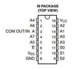
Figure 4-1. Pin Diagram (SOIC) Package
