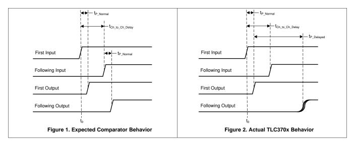
Figure 1 shows expected comparator behavior when one channel transitions slightly before another channel. Both outputs should be delayed only by the normal, specified propagation delay period  $(t_p)$  without any influence from the other channel.
