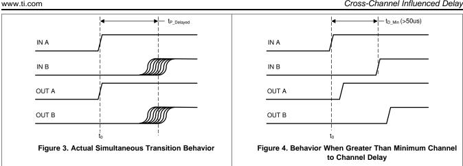
Actual delays depend on supply voltage and the channel to channel delay time, with 16V supply voltage being the worst. At the minimum supply voltage (3V or 4V), the delay may not even be noticeable for all except the most time-critical or jitter sensitive applications.
