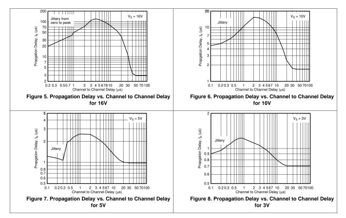
In addition, a single channel can affect itself if the toggle rate is fast enough (time period is less than 50µs). This will be seen as an increase in propagation delay as the toggle frequency period approaches the minimum delay time. The result being a constant output delay period with a jittery trailing end.
