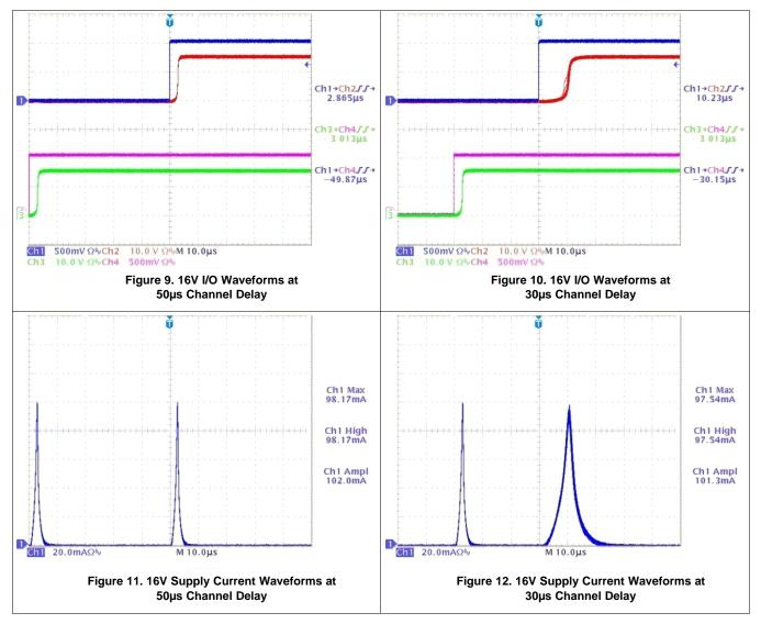
Figure 9 and Figure 11 show the "Normal" output waveform and supply current spikes with a 50µs delay between channels. Each channel has a propagation delay of about 3µs, which is typical for a full 16V output swing.
