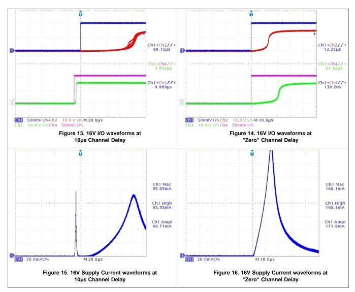
Figure 13 and Figure 15 show a more pronounced effect at a channel-to-channel delay separation of  $10\mu s$ . The "S" shaped output is more pronounced and the channel A propagation delay has extended out to  $80\mu s$ . The "leading" channel B prop delay still remains at  $3\mu s$ .
