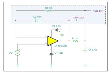
Figure 19: Dual feedback introduced to correct for gain error
