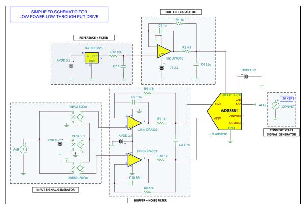
Figure 20: TINA-TI Schematic for Reference Drive and Input Drive
