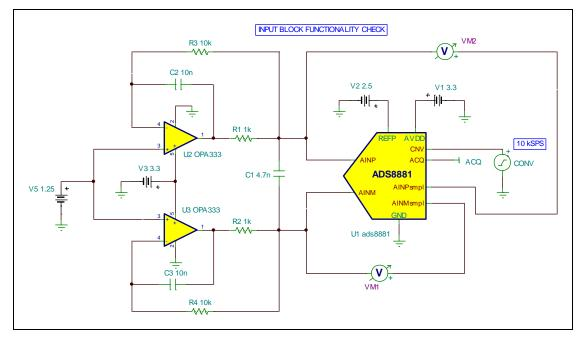
Figure 27: Simplified schematic to check working of input drive
