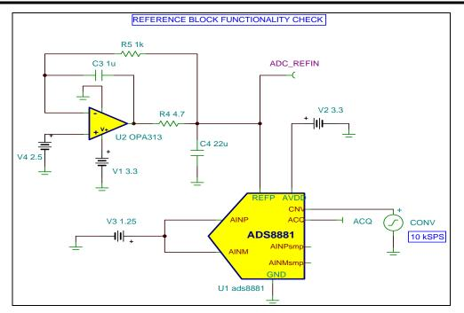
Figure 23: Simplified schematic to check working of reference capacitor
