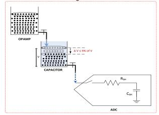
Figure 10: Fly-wheel capacitor delivering charges to C<sub>SH</sub>
