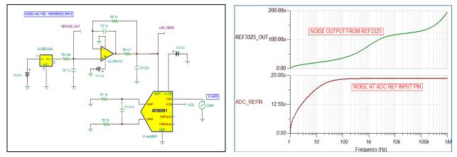
Figure 30: Noise analysis for reference drive
