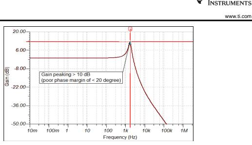
Figure 14: Gain plot – OPA313 with 1 Ohm isolation resistor
