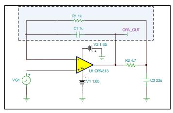
Figure 17: Dual feedback – OPA313 with 4.7 Ohm isolation resistor
