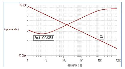
Figure 13: Crossover between the output impedance of OPA333 and 22uF capacitor
