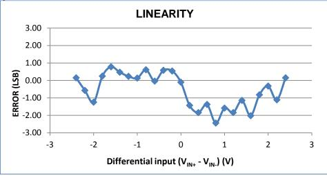
Figure 35: 25 point linearity check
