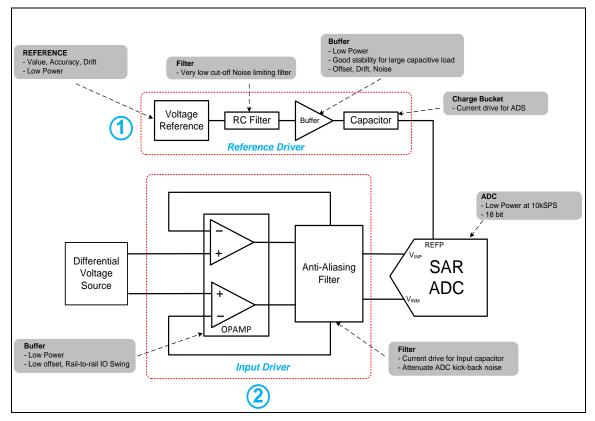
Figure 2: Reference and Input drive circuit elements for low power
