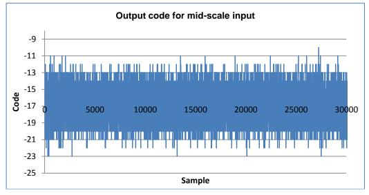
Figure 33 : Output code for mid-scale input
