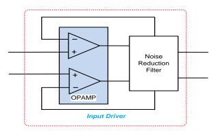
Figure 11: Buffer driving the input
