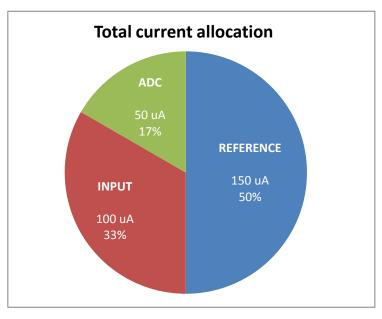
The remaining 150 uA is shared between the input driver (100 uA) and ADC (50 uA).
