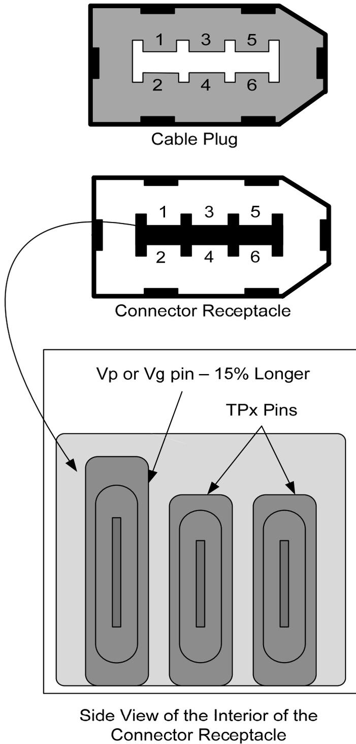
**Figure 1. 1394 6-Pin Receptacle (Connector) and Plug (Cable) Diagrams**
