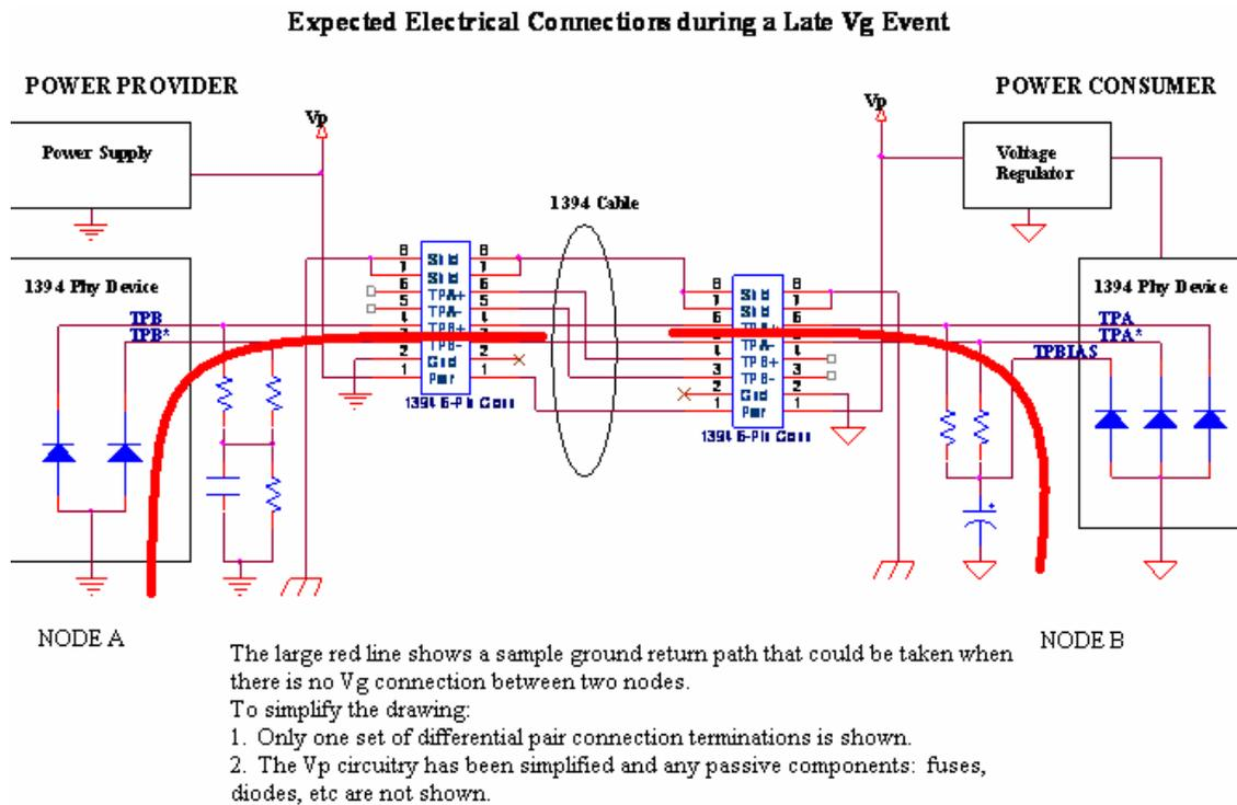
**Figure 5. Late Vg Electrical Connections**
