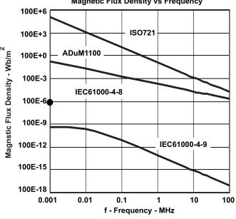
Magnetic Flux Density vs Frequency
