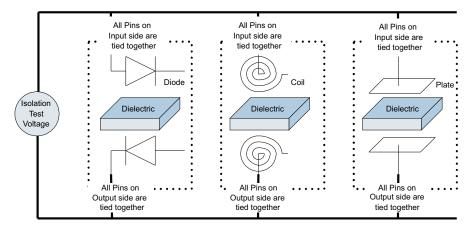
Figure 10. Two-Terminal Isolation Voltage Test
