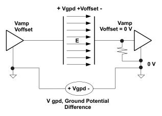
Figure 8. Capacitive Coupling
