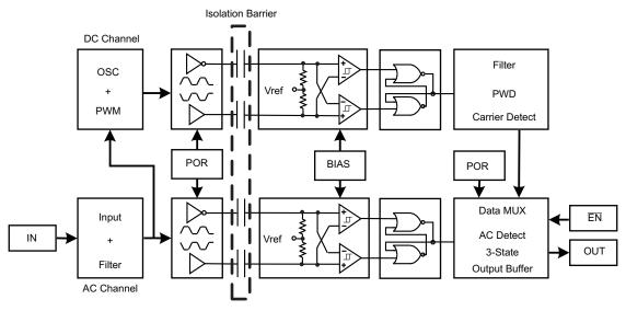
Figure 9. ISO72x and ISO72xM Block Diagram
