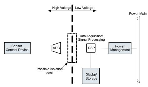
Figure 2. Isolation Between High-Voltage and Low-Voltage Circuits
