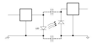
Figure 11. Barrier Capacitance
