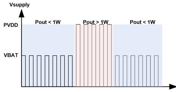
Figure 5-1. Y-Bridge Modulation
