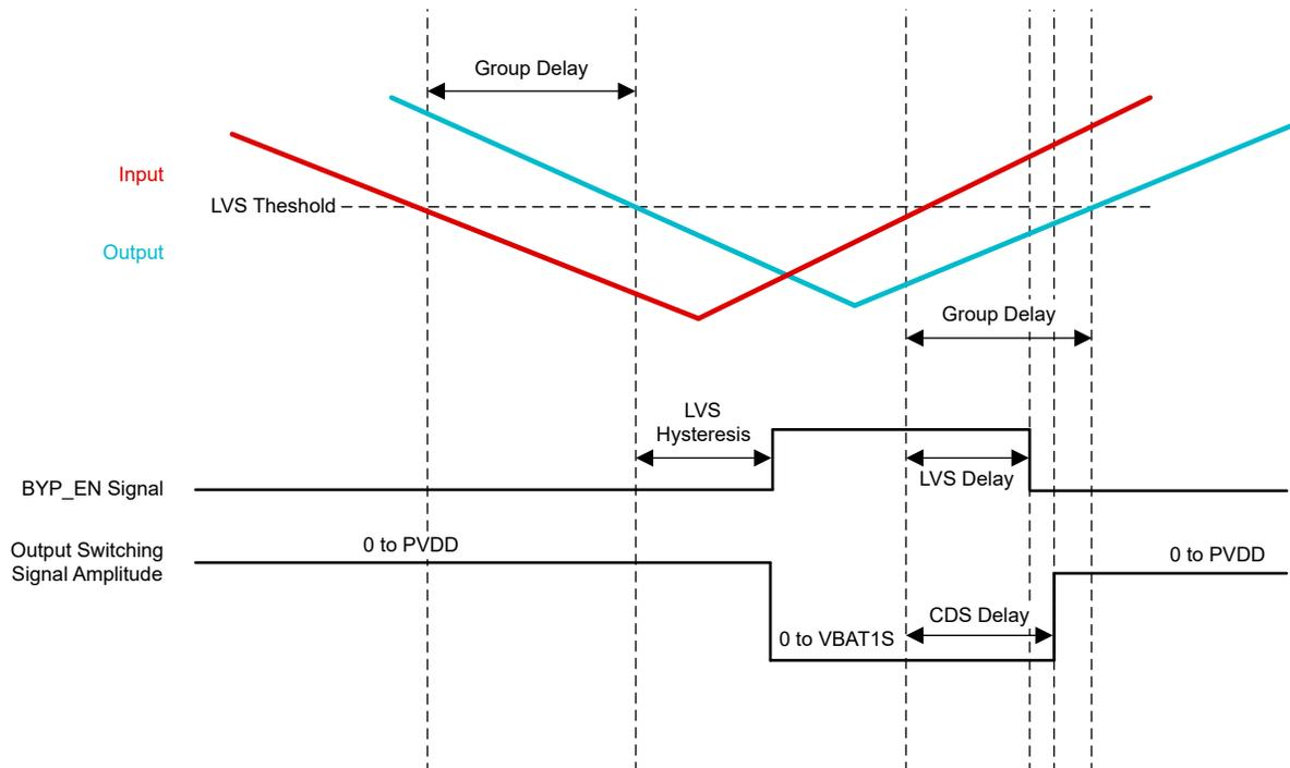
Figure 4-1. Low Voltage Signaling Thresholds and Delays
