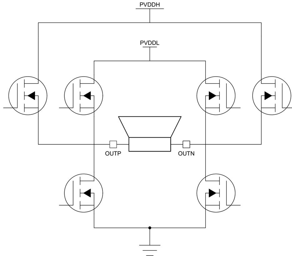
**Figure 2-2. Simplified Y-Bridge Schematic**
