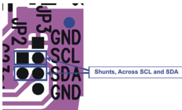
**Figure 1. Place Shunts Horizontally Across SCL and SDA**
