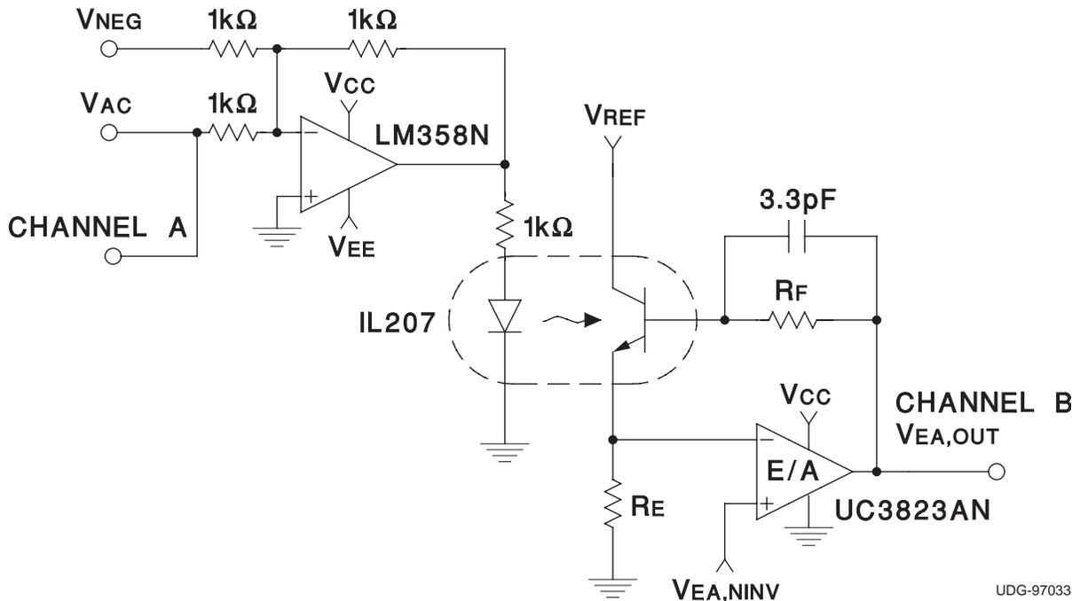
**Figure 8. Circuit Used in Tests 5 through 9**
