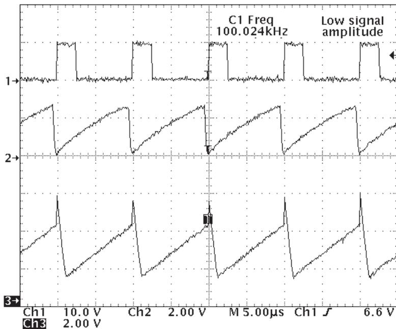
Figure 5. UCC3802 Oscillator Waveform with Synchronization
