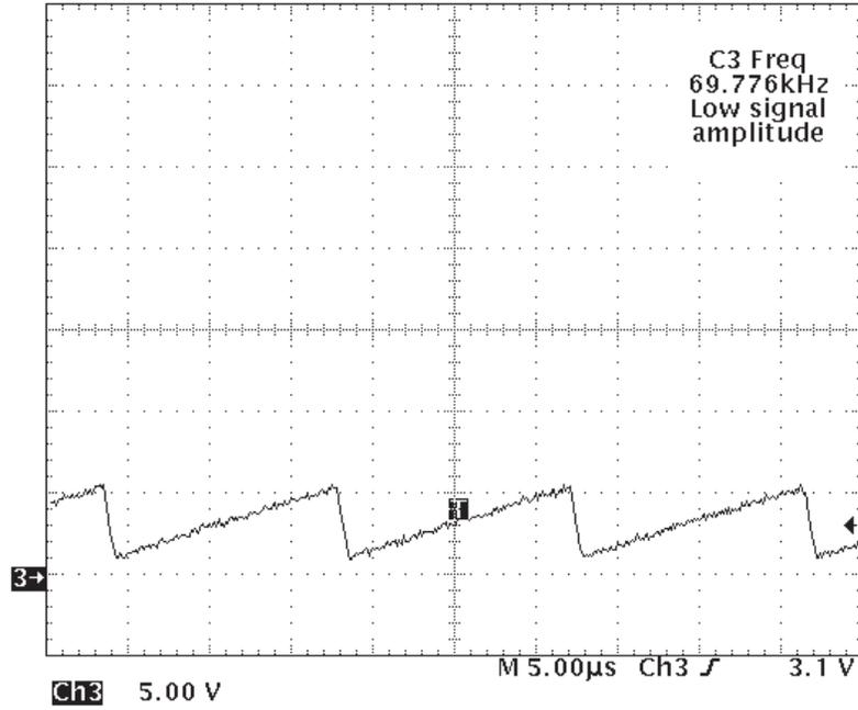
Figure 4. UCC3817 Oscillator Waveform Without Synchronization
