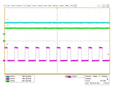
Figure 12. Steady State Waveform / Constant Voltage Charging ( $V_{IN}$  = 12 V,  $V_{OUT}$  = 3.5 V,  $I_{OUT}$  = 2 A)
