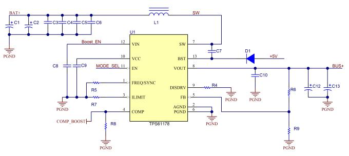
Figure 3. Charging Circuit
