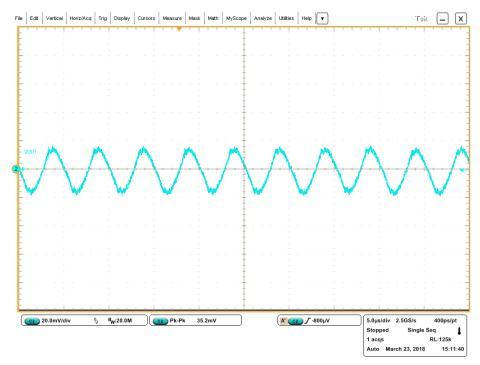
Figure 14. Output Voltage Ripple / Constant Voltage Charging (V<sub>IN</sub> = 12 V, V<sub>OUT</sub> = 4.2 V, I<sub>OUT</sub> = 6 A)
