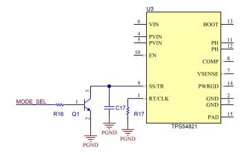
Figure 10. Enable Buck Circuit
