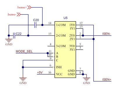
Figure 5. Analog Switch Circuit
