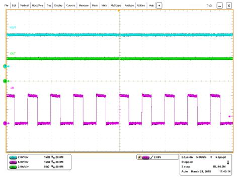
Figure 11. Steady State Waveform / Constant Current Charging ( $V_{IN}$  = 12 V,  $V_{OUT}$  = 4.2 V,  $I_{OUT}$  = 3 A)
