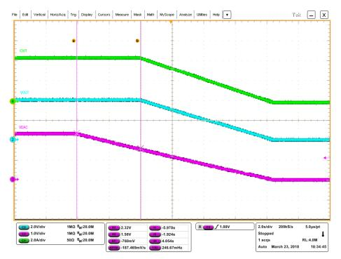
Figure 17. Transition from a Constant Voltage Charging to a Constant Current Charging
