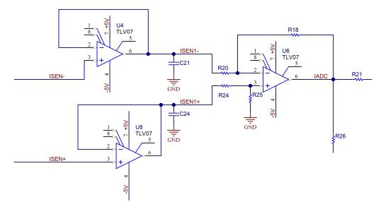
Figure 6. Voltage Conditioning Circuit
