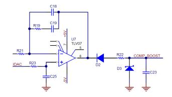
Figure 7. Compensation Circuit
