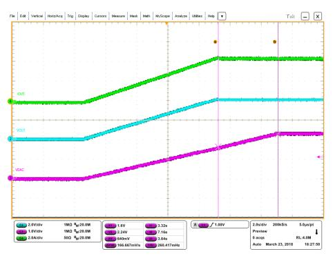
Figure 16. Transition from a Constant Current Charging to a Constant Voltage Charging
