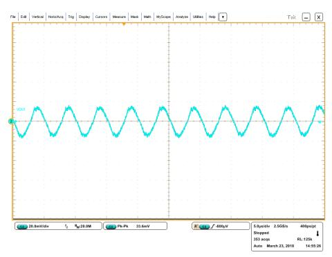
Figure 15. Output Voltage Ripple / Constant Current Charging (V<sub>IN</sub> = 12 V, V<sub>OUT</sub> = 4.2 V, I<sub>OUT</sub> = 6 A)
