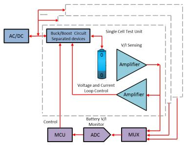
Figure 1. Separation Solution Block Diagram
