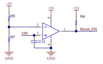
Figure 9. Battery Over-Discharge Protection
