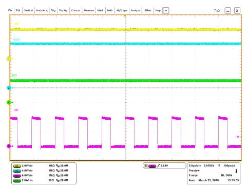
Figure 13. Steady State Waveform / Constant Current Discharging (V<sub>IN</sub> = 4 V, V<sub>OUT</sub> = 12 V, I<sub>OUT</sub> = 3 A)
