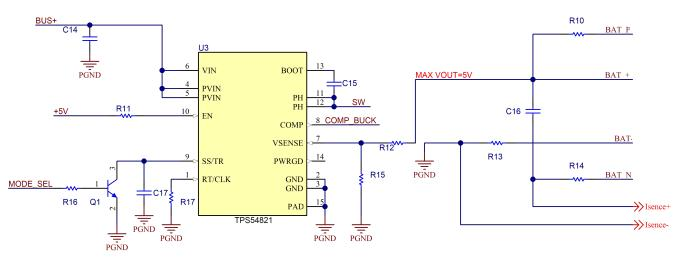
Figure 4. Discharging Circuit
