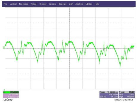
6.4 3.3V<sub>ripple</sub> with loads 20V/50mA, 5V/10mA, 4V/1.4A, and 3.3V/50mA:
