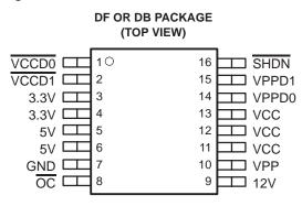
Figure 3. TPS2211 16-Pin SSOP Package
