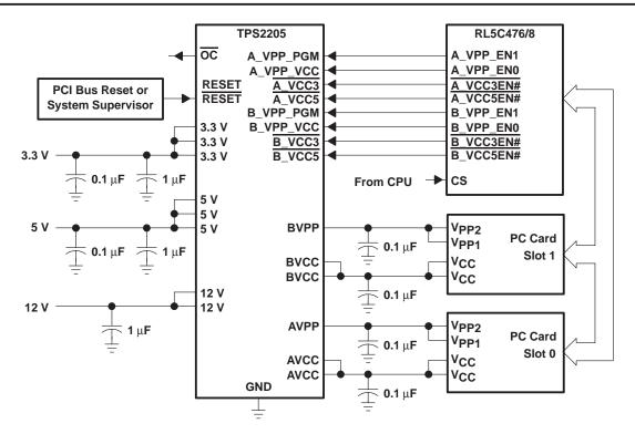
Figure 5. TPS2205 and Ricoh RB5C478 Application
