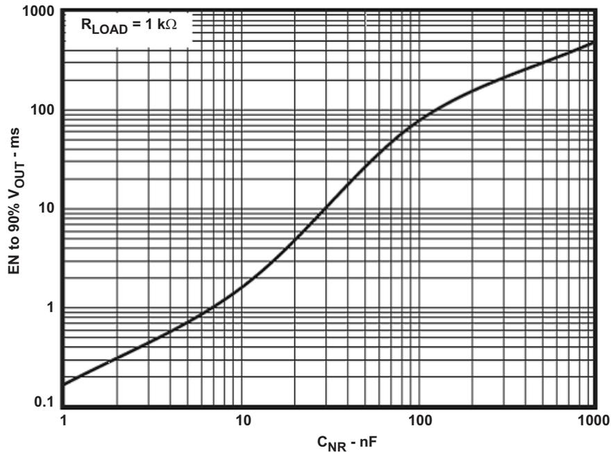
Figure 4. LDO Start-Up Time vs Noise Reduction Capacitor
