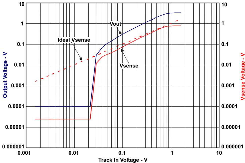
Figure 2. Relationship Between Tracking Voltage and Output Voltage
