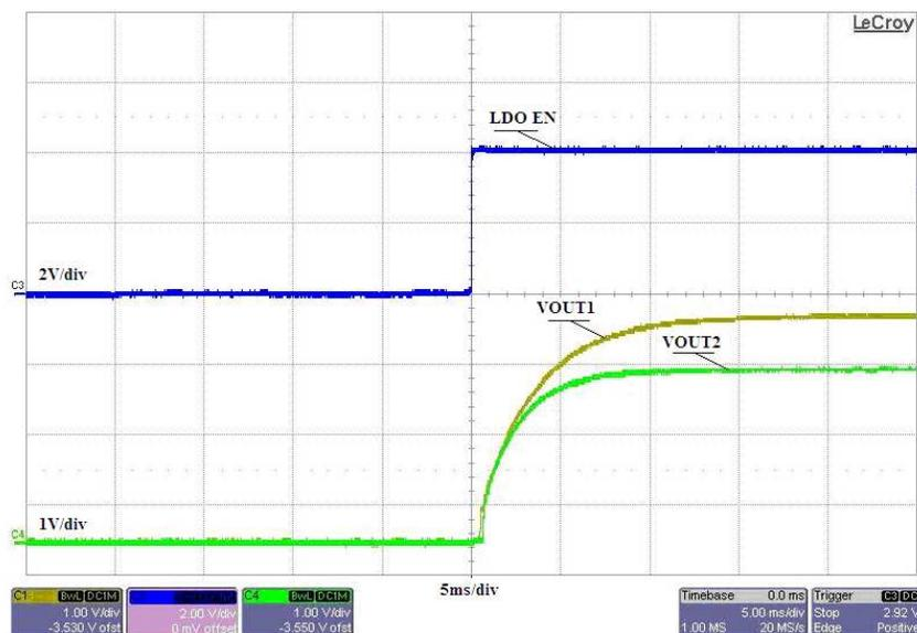
**Figure 12. Ratiometric Start-Up Result of Circuit in [Figure 11](#)**
