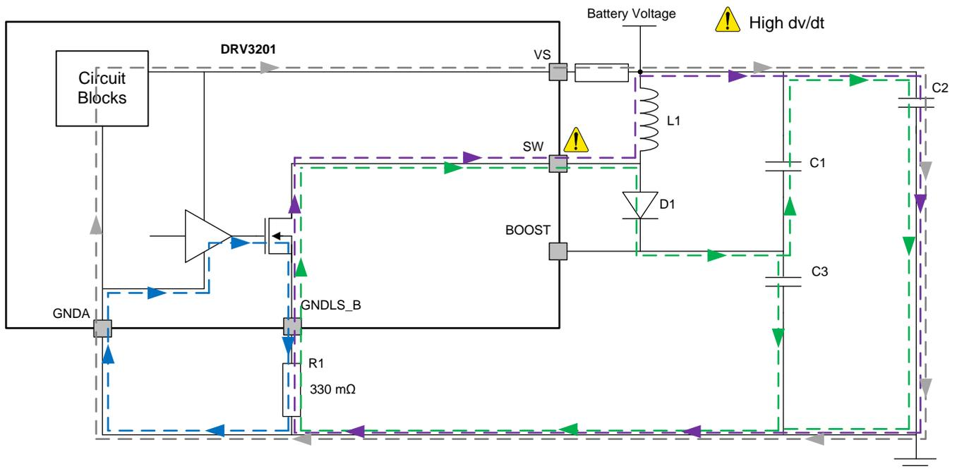
**Figure 7. High Switching Transient Current Return Paths**
