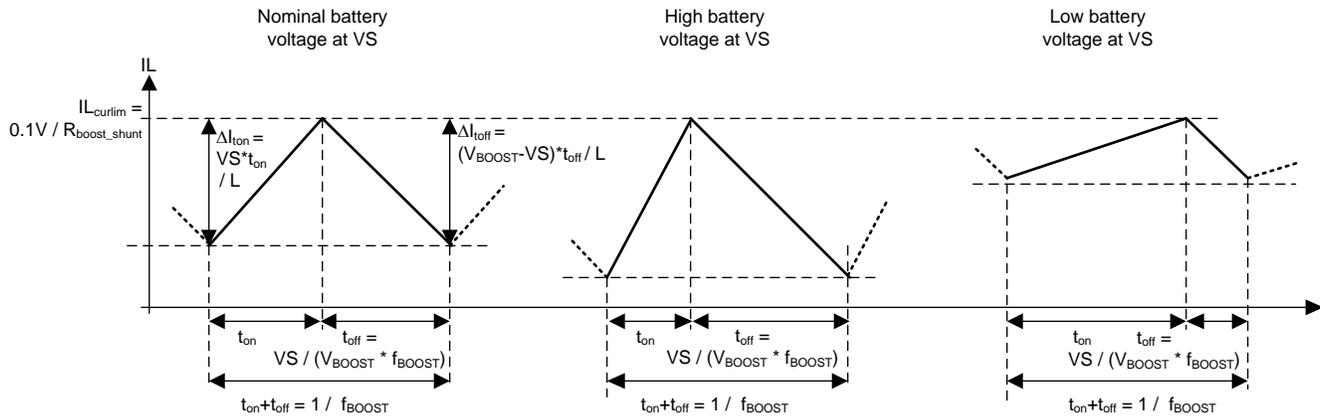
**Figure 1. Coil Current Waveforms in Steady State for Nominal, High and Low Battery Voltage**
