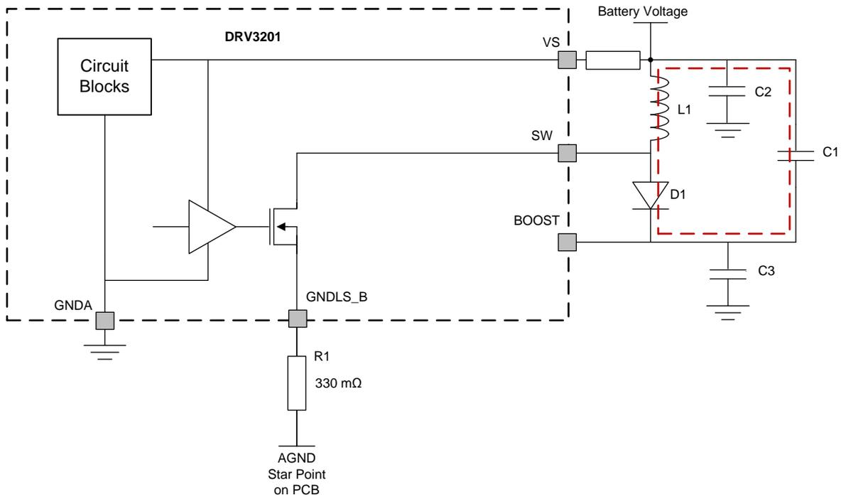
Figure 6. High Current Path During Boost FET 'Off' State
