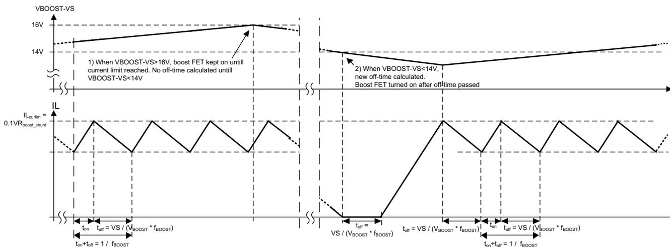
Figure 2. Boost Waveforms Showing Burst Pulsing Controlled by Hysteretic Comparator Levels
