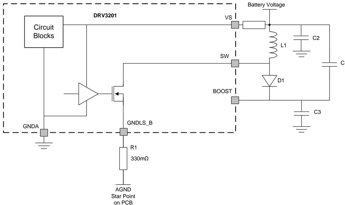
Figure 3. Recommended Application Circuit for Boost Converter
