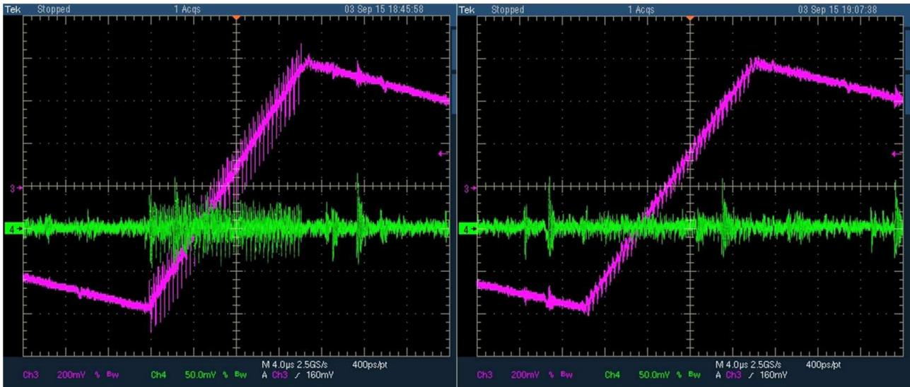
**Figure 4. Boost Output and Current Sense O1 Output, Before and After Bypass Capacitor**
