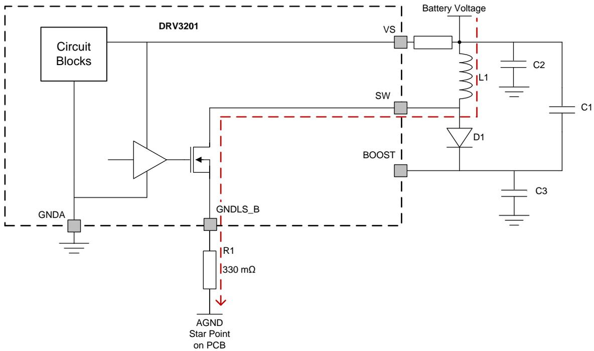
Figure 5. High Current Path During Boost FET 'On' State
