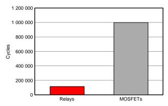
Figure 9. Switching Cycle Comparison
