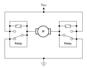
Figure 3. H-Bridge Control of BDC Motor Using Relays
