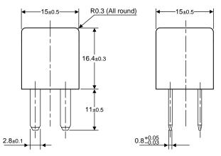
Figure 10. Typical Relay Dimensions
