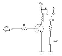
Figure 8. Relay Interface Circuit With MCU
