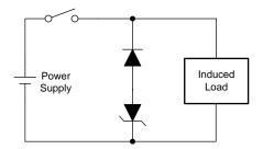
Figure 5. Suppression Circuit for High-Voltage Transients
