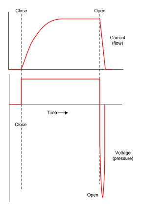
Figure 6. Relay Switching Time and High-Voltage Breakdown
