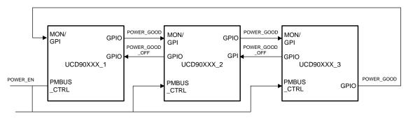
Figure 14. POWER\_GOOD and POWER\_GOOD\_OFF Cascading
