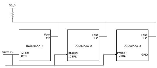
Figure 15. Fault Pin Cascading
