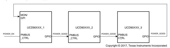
Figure 12. POWER\_GOOD Cascading Case 1
