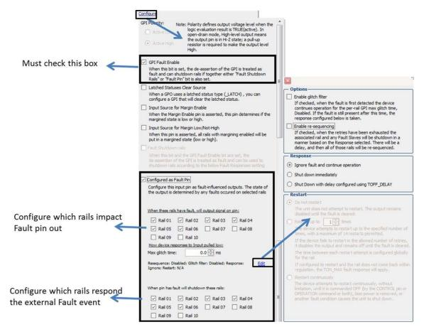
Figure 9. Fault Pin Configuration for UCD9090A and UCD90160A
