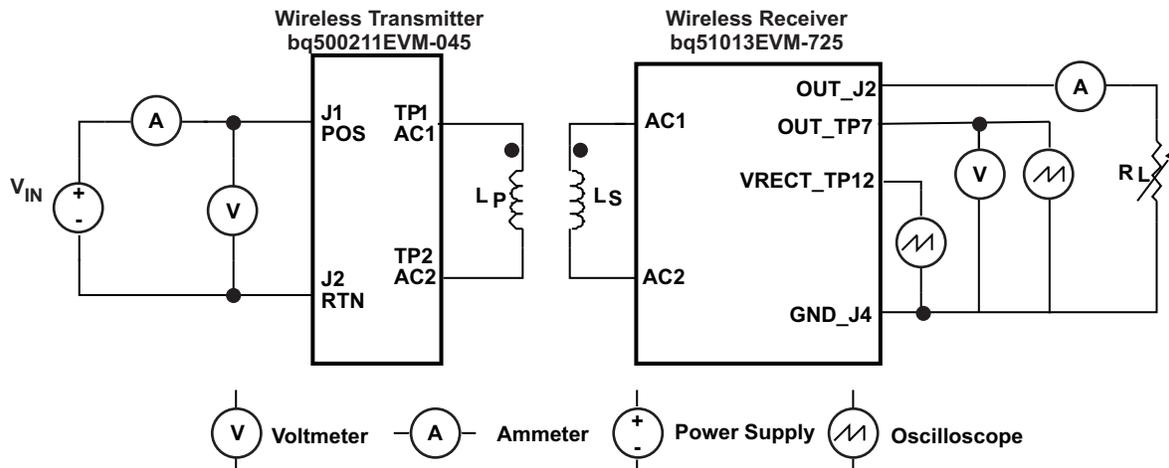
**Figure 4. Equipment Setup**
