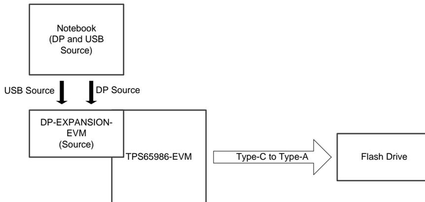
**Figure 5. Connecting EVM to Type-A Device**
