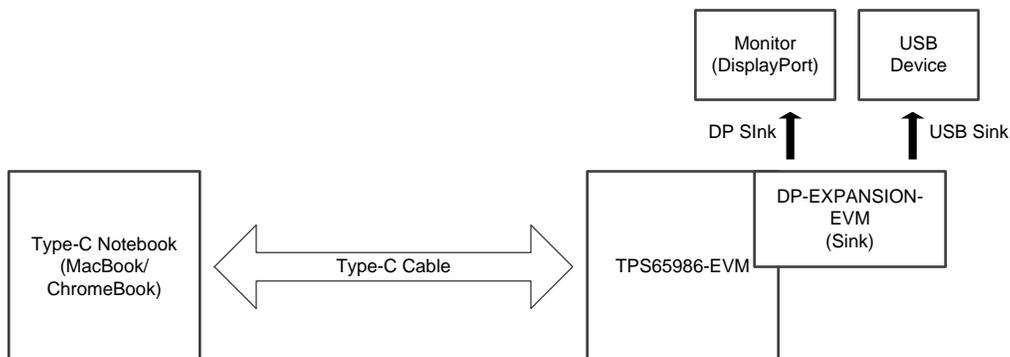
**Figure 8. Connecting EVM to Type-C Host**
