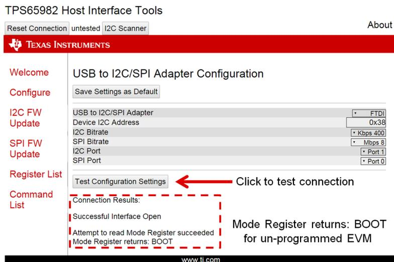
**Figure 14. Host Interface Adapter Configuration Test (Error-Free Results)**
