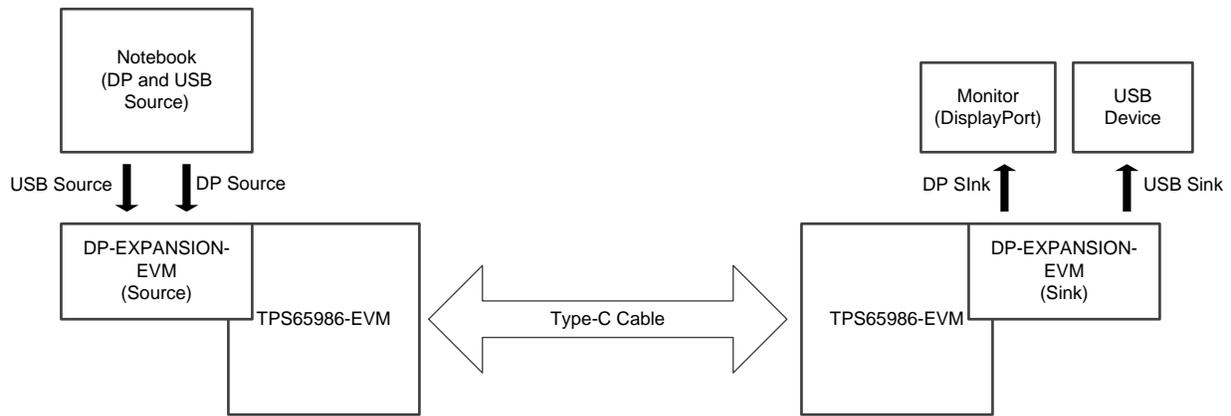
**Figure 6. Connecting EVM to EVM for Type-C System**
